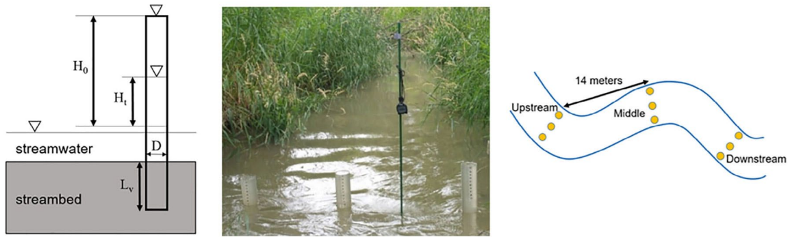
Figure 3 Basic design of falling-head permeameter test. Left : Schematic of the field permeameter. Middle : Photograph of permeameters with each tube installed to depth of 30 cm. Right : Layout of three transects along the stream for each site.
