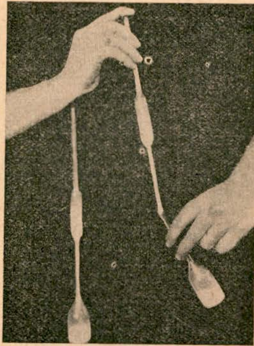
FIG. 2.—Two methods of transferring the milk to test bottle.
