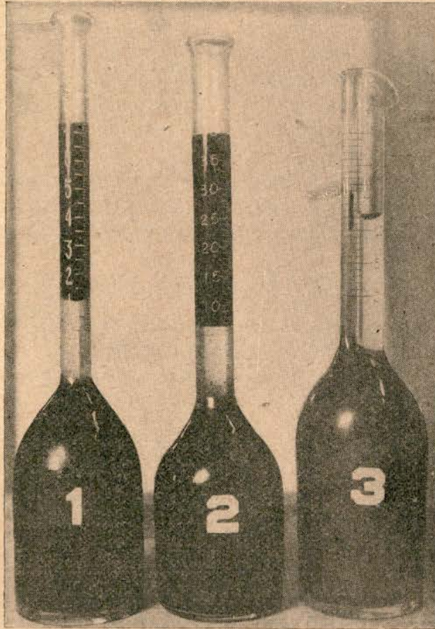
Fig. 10.—1. Completed whole milk test. 2. Completed cream test. 3. Completed skim milk test.
