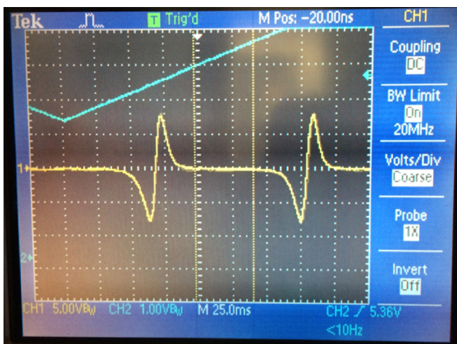
Fig. 12. Output of mixer circuit. The top trace is the cavity PZT ramp while the bottom trace is the mixer output. There are two error signals in the output, representing two different resonant modes of the cavity.
