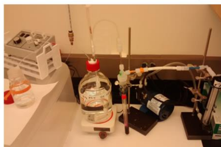
Fig. S2. Purge and trap method following sample digestion. Approximately 1 L of digested water was placed in a 2 L acid-cleaned borosilicate media bottle with a Corning three-hole delivery cap. The 10% \text{SnCl}_2 reductant was continuously and slowly added to the stirred solution to reduce \text{Hg}^{2+} (aq) into \text{Hg}^0 (g). A vacuum directed the reduced \text{Hg}^0 (g) into a 1% \text{KMnO}_4 trap solution that oxidized \text{Hg}^0 (g) to \text{Hg}^{2+} (aq), and trapped Hg was later analyzed using CVAFS to determine “purge and trap” recovery as well as analyzed using MC-ICP-MS for determining Hg stable isotope ratios in the sample.
