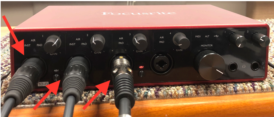
Figure 3.10. Front of Interface with Microphone Connects
