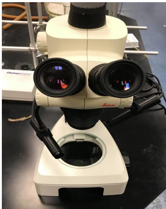
Figure 6. Leica L2 Stereomicroscope used for sample preparation and sex identification. Under the stage is a mirror that reflects the light to the bottom of the sample.
