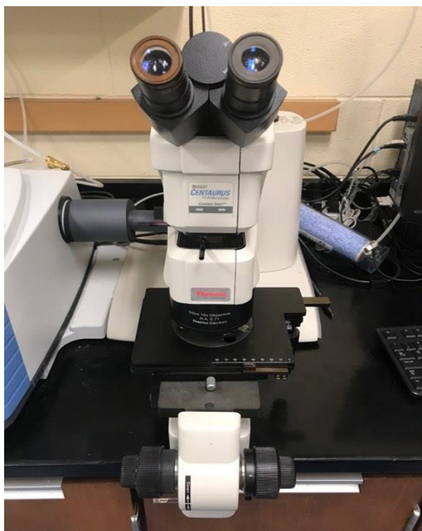
Figure 5. Photo of ThermoNicolet™ model Centaurus IR microscope used to make all spectroscopic measurements.
