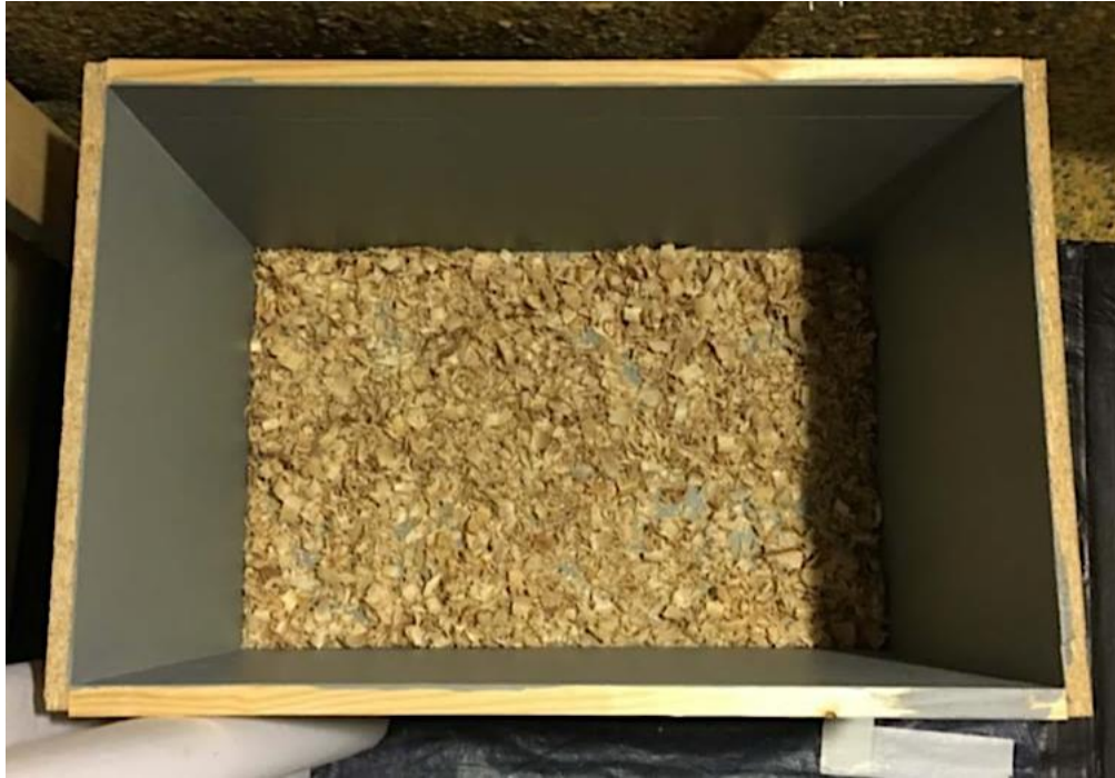
Figure 3. The 63 X 42 X 45 cm (w X d X h) wooden box with aspen bedding on the floor for the social preference task (SPT).
