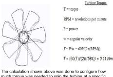
The calculation shown above was done to conligure now much torque was needed to spin the turbine at a specific angular velocity. Although this calculation alone is not beneficial, it was necessary in order to calculate other design parameters of the product, such as the turbine radius and generator power output. This is just a sample of the design calculations that were done in order to create the product and the circuit within the product, which can be seen below.
