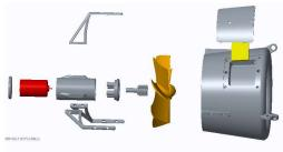
The figure above is a disassembled view of the final product in which had a low reproduction cost due to the utilization of 3D printing most of the parts. These parts were printed using ABS to ensure that they would not degrade and pollute the water source while the PHG is being used.
