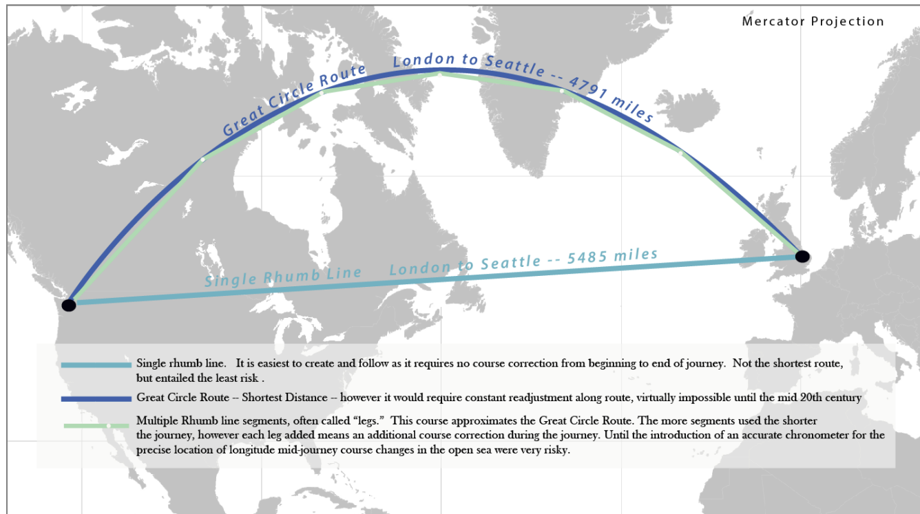
Figure 2.7. A Great Circle Route Compared to the Rhumb Line and Multiple Rhumb Lines.
