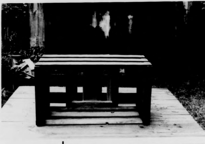
Figure 3. Melon crate with end piece used as reinforcement.
