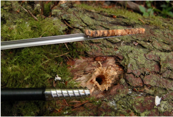
Figure 6. Haglof Increment Borer Used to Collect Core Samples.
