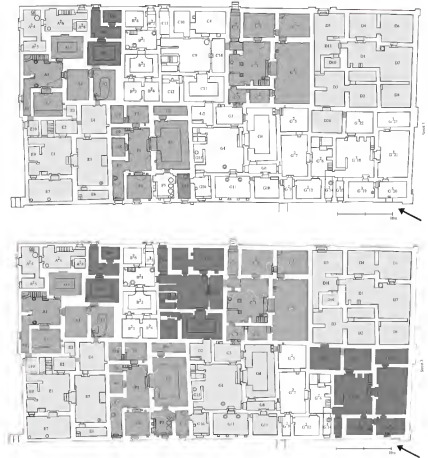
Figure 14.3: Plan of C7 showing courtyard-based units (above) and intercommunicating units (below). After Henry Pearson's original in the Dura-Europos archives at the Yale University Art Gallery (plan by the author)
