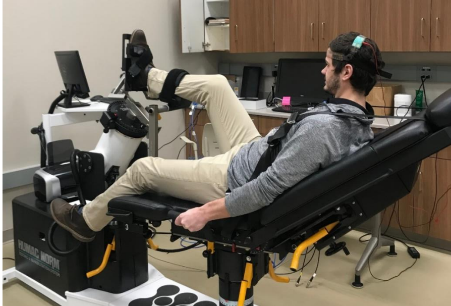
Figure 6. A side view of the set up on the dynamometer and the aTDCS electrodes inside of the green sponge above the hotspot.
