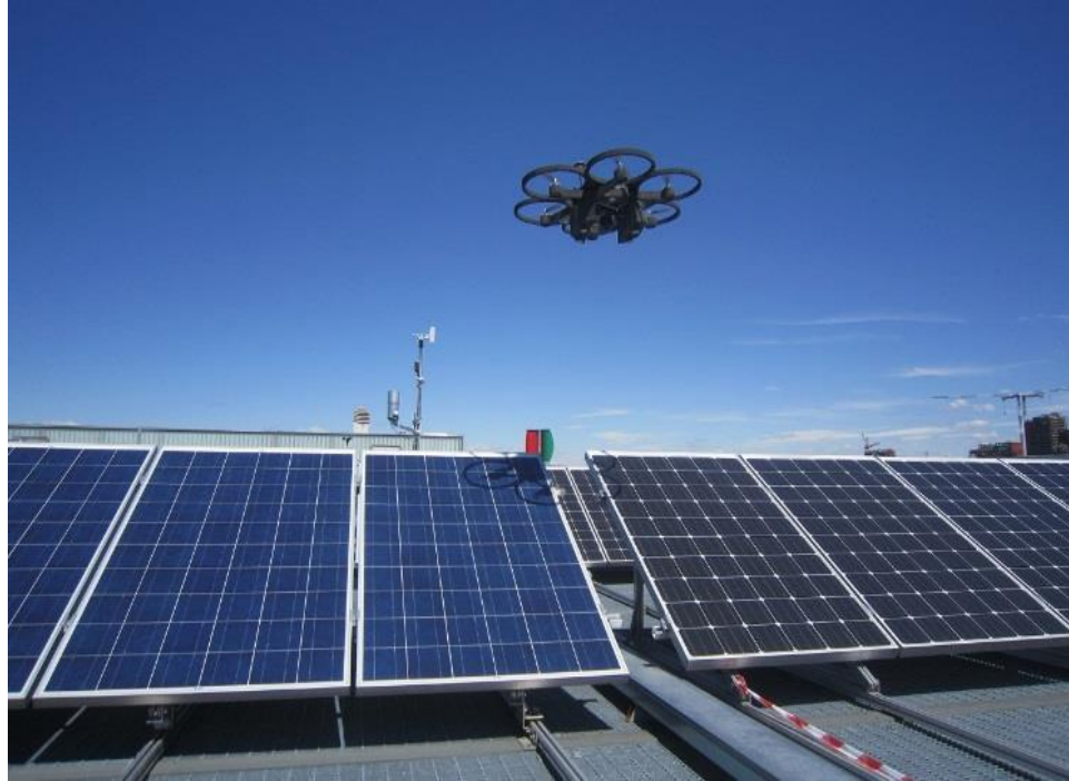
(Figure 1) This photo shows a drone with an IR camera connected inspecting a group of solar panels. This particular PV farm is located on the top of a car garage. This image depicts just how versatile and easy to manage drones are. This further shows why drones are the most efficient inspection method. (Aghaei, 2014)
