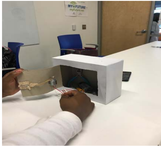
Figure 56. The Mechanics in the Toy Safe. The Picture Shows the Popsicle Sticks and Rubber Band Attached to the Motor, which Served as the Locking and Unlocking Component of the Toy Safe.
