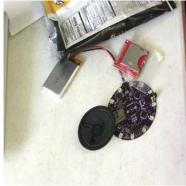
Figure 8. The Arduino the Girls Used to Program the Music as an MP3 File. A Small Memory Card is Placed on the Arduino, Which Enables Music to Be Played.
