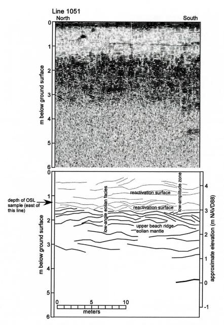
Figure 4. Processed ground penetrating radar data (top) and line interpretation (bottom) illustrating low-angle, mounded dune facies.
