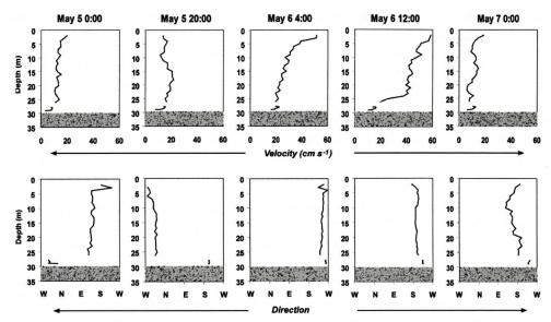
Figure 5. Current magnitude and direction profiles throughout the May 2005 Northerly wind event at Site 2. Velocities above 4 mab were measured by the ADCP and velocities within the bottom boundary layer were measured by the PC-ADP. Profiles appear to be more continuous between the upper and lower water column when the instrument frame was 1km away from the hardbottom reef. Times denoted by arrows in Figure 4.
