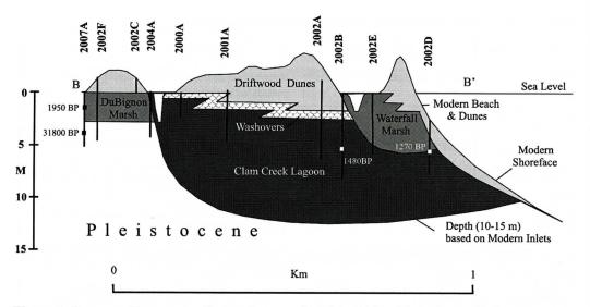
Figure 5. Cross-section across the northern end of Jekyll Island (see figure 4) showing abandoned inlet infilled by lagoonal clays.
