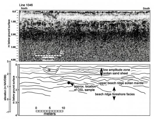
Figure 3. Processed ground penetrating radar data (top) with a line interpretation (bottom) revealing a lower beach ridge unit consisting of seaward (south) dipping reflections, with hummocky bedding, and an upper eolian sand sheet unit.
