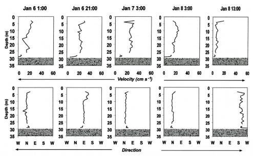
Figure 7. Current magnitude and direction profiles throughout the January 2002 Southerly wind event at Site 1. Velocities above 4 mab were measured by the ADCP and velocities within the bottom boundary layer were measured by the PC-ADP. Magnitude and direction profiles appear to be less continuous between the upper and lower water column when currents are flowing from south to north, towards the hardbottom reef. Times denoted by arrows in Figure 6.
