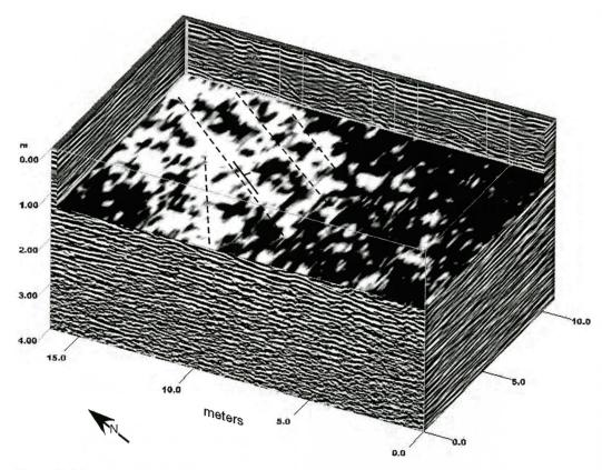
Figure 7. 1.2 m depth slice at Site 6. The orientation is indicated by the north arrow at the bottom of the figure. White indicates high amplitude reflections. Dashed lines emphasize the strike of the clinoforms (NNE), which dip to the east-southeast and indicate sediment transport from the west.
