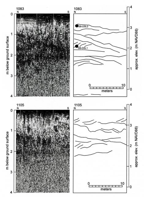
Figure 6. Processed GPR lines 1083 (top) and 1105 (bottom) from Site 6. Processed data are shown on the left, and a line interpretation is shown on the right.
