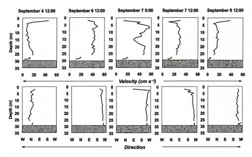
Figure 3. Current magnitude and direction profiles throughout the September 2000 Northerly wind event at Site 1. Velocities above 4 mab were measured by the ADCP and velocities within the bottom boundary layer were measured by the PC-ADP. Profiles appear to be discontinuous during the event when currents are flowing over the hardbottom located north of the instrument frame. Times denoted by arrows in Figure 2.
