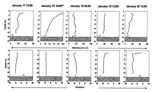
Figure 9. Current magnitude and direction profiles throughout the January 2006 southerly wind event at Site 2. Velocities above 4 mab were measured by the ADCP and velocities within the bottom boundary layer were measured by the PC-ADP. Profiles appear to be more continuous between the upper and lower water column when the instrument frame was 1km away from the hardbottom reef. Times denoted by arrows in Figure 8. \*\* Note change in scale.
