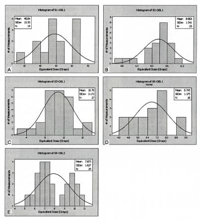
Figure 8. Frequency distribution histograms of Equivalent Dose –  $D_e$  (Grays). The age of the sample is calculated by dividing the De by the dose rate (Gy/ka) (see Table 2).
