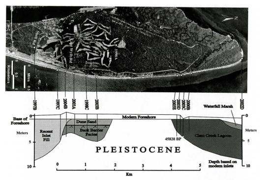
Figure 6. Longitudinal section based on vibracores along Jekyll beach. The section shows Clam Creek inlet to the north and old 'Jekyll' inlet to the south separated by a core of Pleistocene substrate.
