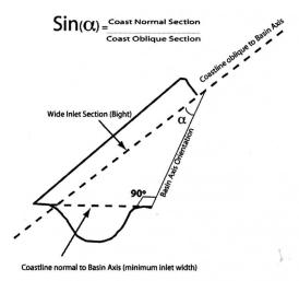
Figure 4. Sketch illustrating the sectional width produced by the relationship between coast-line orientation and the axis of coastal basins. Large angles between coastlines and basin axes produce narrow sections. Near parallel, oblique angles between coastlines and basin axes produce very wide sections.
