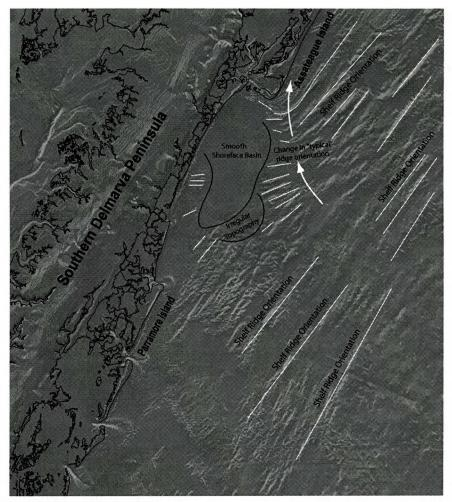
Figure 5. Shaded highlighted relief image of the middle Atlantic shoreface in and adjacent to the Chincoteague Bight. The image reveals the extensive coverage of the inner shelf by linear sand ridges that are slightly oblique to the coastline. Curved ridges and steeper ridge angle occur at the margin of a topographically smooth area of the shoreface.
