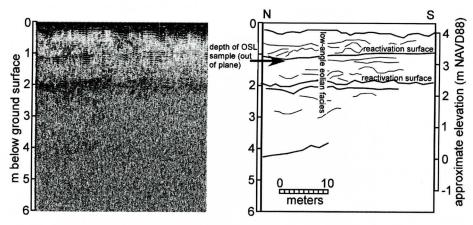
Figure 5. Site 3 - Processed ground penetrating radar data (left) and line interpretation (right).
