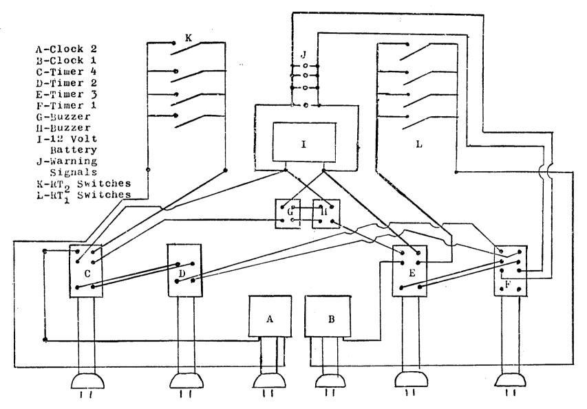
Figure 3. Non-technical schematic of wiring.
