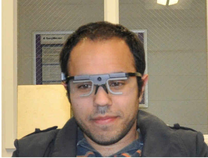
Figure 3.7: Eye Gaze tracking device donned
