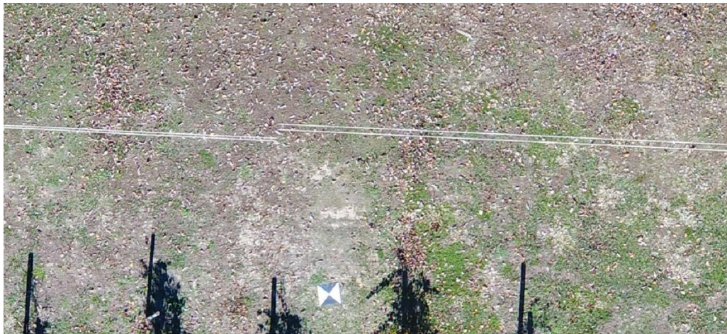
Figure 25. Structure from Motion Flaws Seen in the Misaligned Powerlines.
