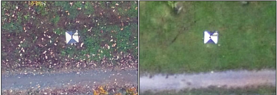
Figure 18. 60-Meter Orthomosaic Images Showing the Difference in Clarity Between the P4P (Left) and P3P (Right) Cameras, Respectively.
