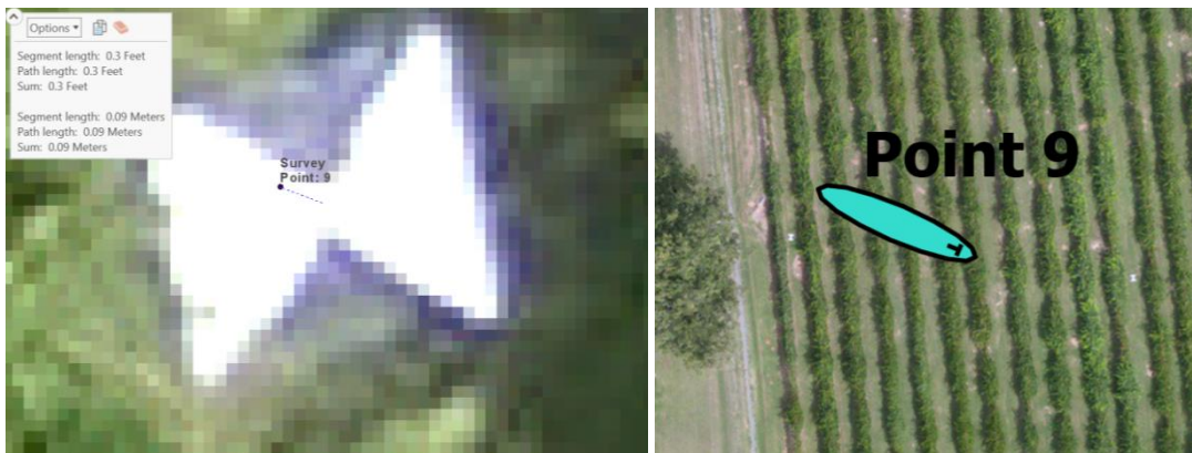
Figure 12. Error Trajectory from Survey Point Nine in ArcGIS Pro Compared to PhotoScan Report, Respectively.
