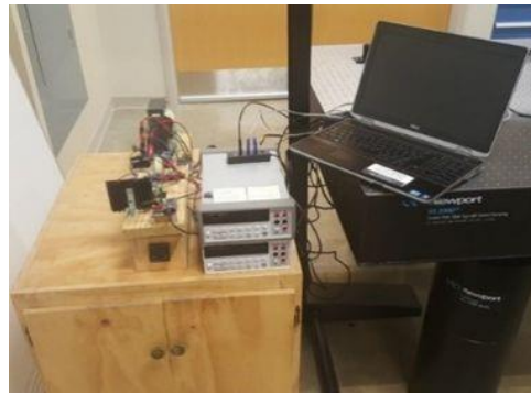
Fig. 3.4: Temperature controlled enclosure and experimental setup
