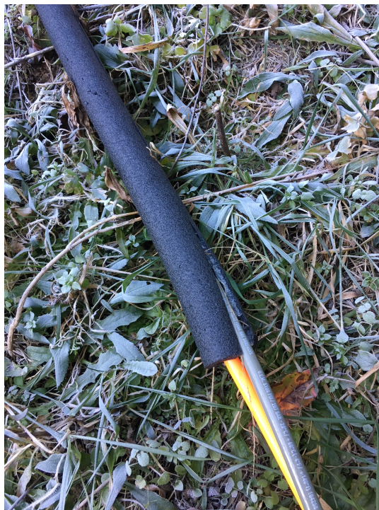
Figure 2. The air and water hoses are placed together in an insulating sleeve so that the heat from the water will prevent the air hose from collecting ice and freezing.
