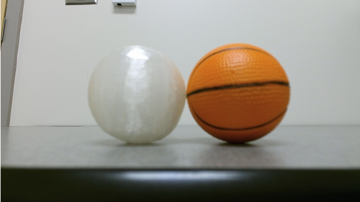
Figure 5.10: Comparison of 3D printed model and original ball
