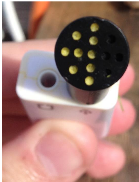
Figure 4.8: Microphone, partially clogged with propolis
