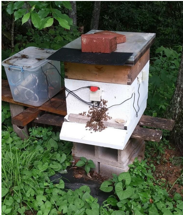
Figure 5.1: A BeeMon prototype with audio and video recording
