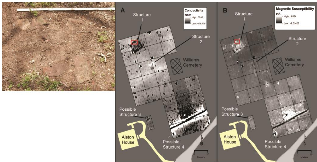
Figure 2.5. Structure One Rubble From Foundation Identified Within Conductivity and Magnetic Susceptibility Images
