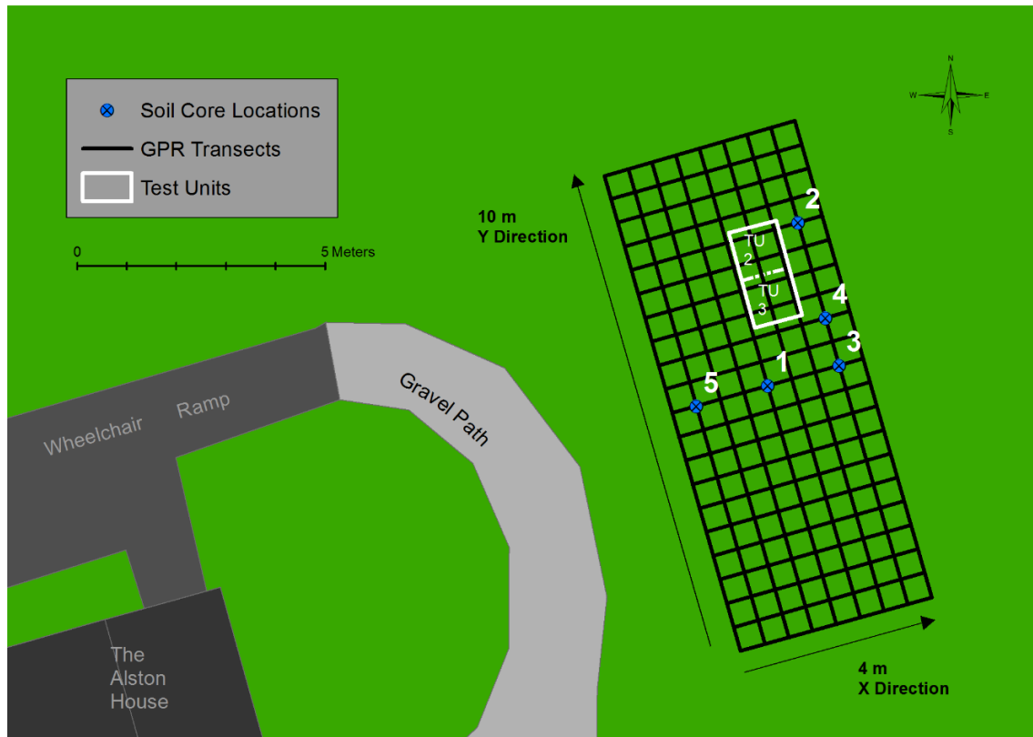
Figure 3.3. GPR Survey Area With Soil Core Sample Locations
