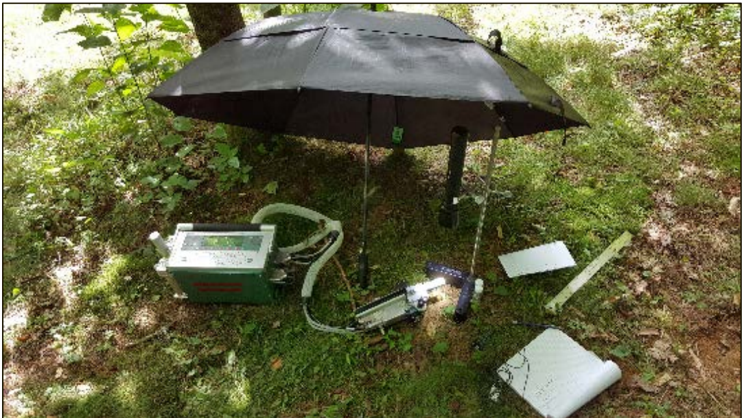
Figure 12. An LED flashlight was used to create lightflecks for photosynthesis measurements.
