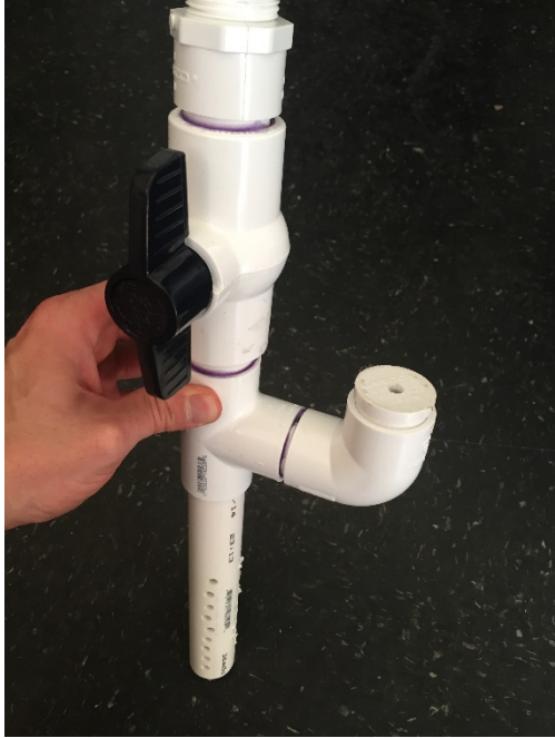
Figure 6. Siphon aeration outlet.
