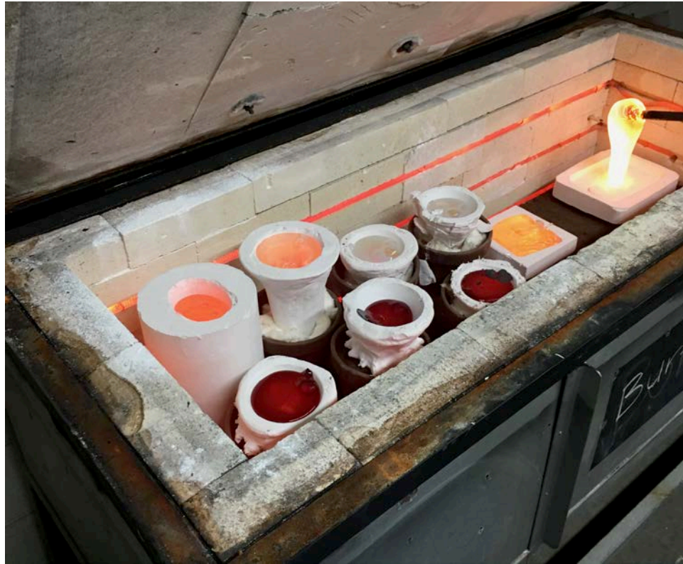
Figure 44. Kiln Casting Glass Process
