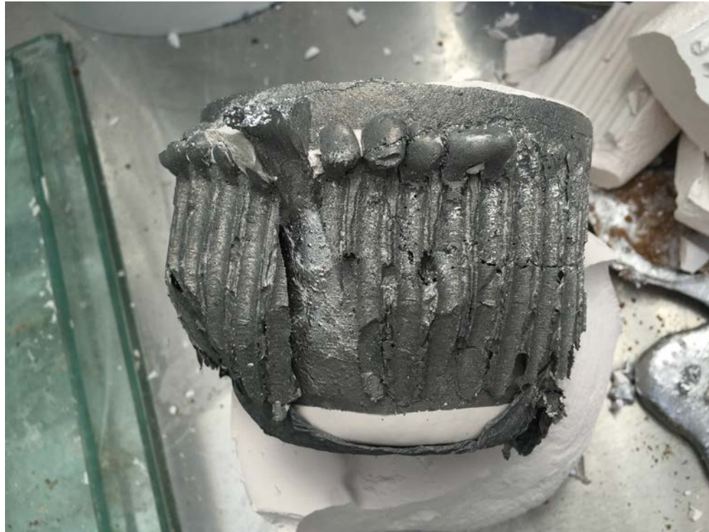
Figure 47. Aluminum Casting Failure
