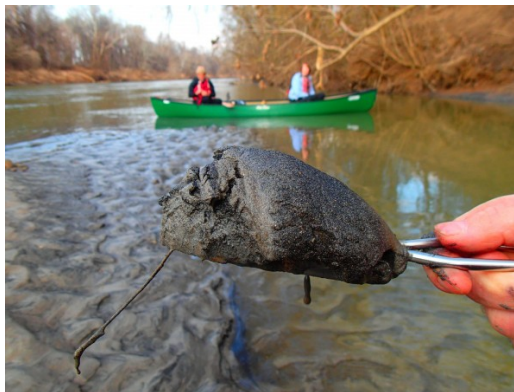
Figure 4- Coal ash sludge pulled from the bottom of the Dan River following the Duke Energy spill (Catanoso, n.p.)
