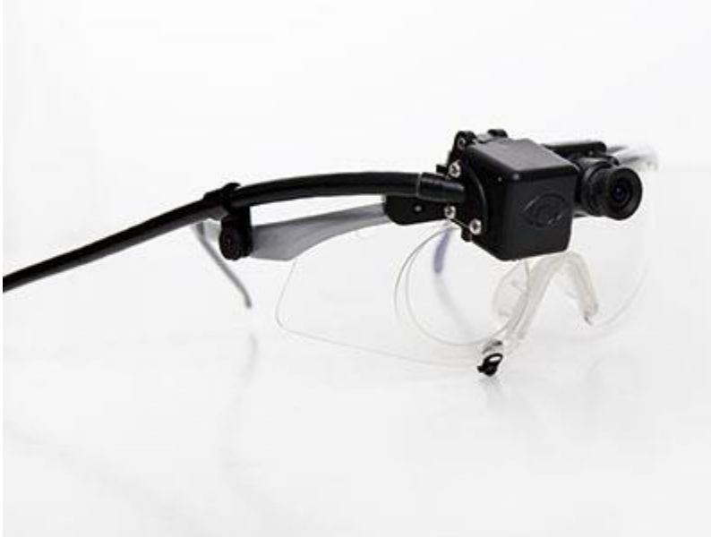
Figure 15. ASL MobileEye Eye Tracking Headset.
