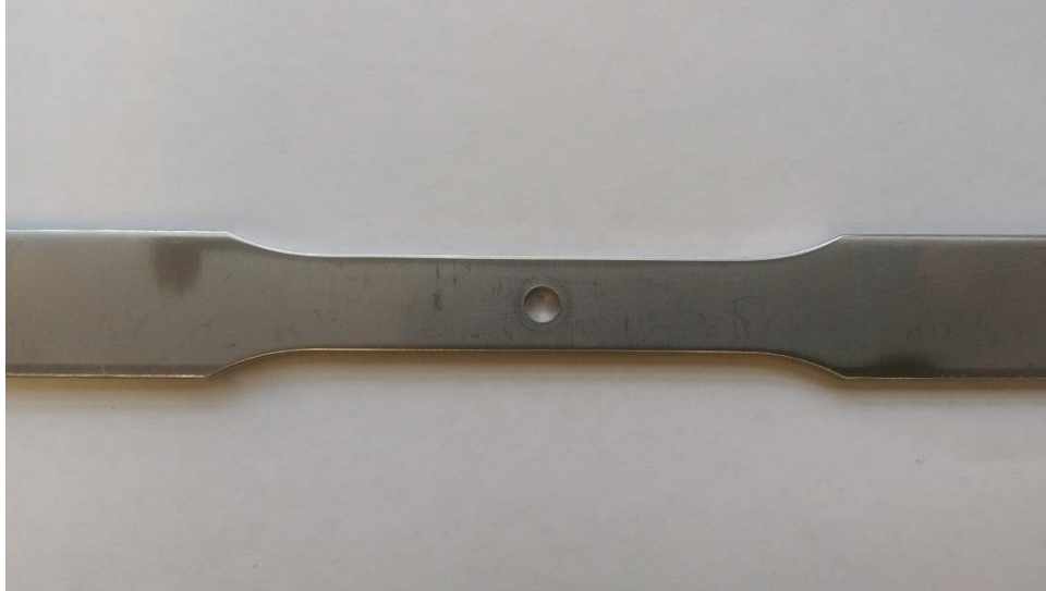
Figure 2-7: Tensile specimen containing a circular hole stress concentration
