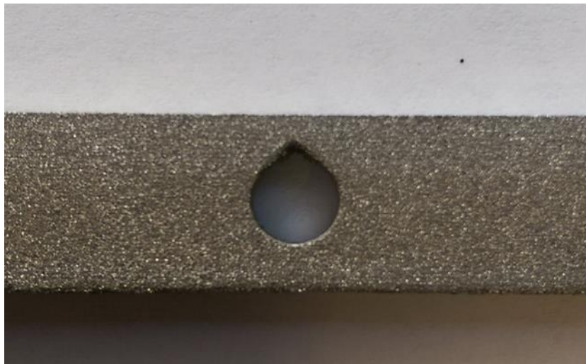
Figure 3-5: Edge oriented test specimen build without stress concentration supports
