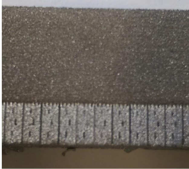
Figure 3-8: Support Material Tooth Structure
