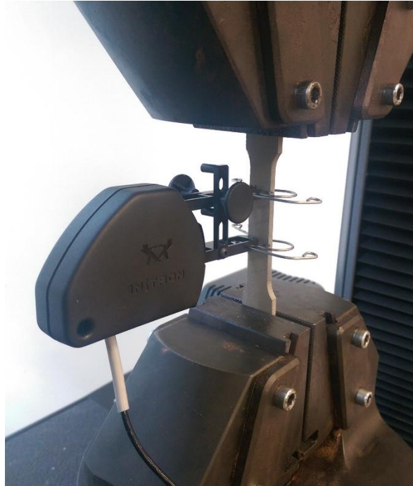
Figure 3-10: Instron Part Test Set-up
