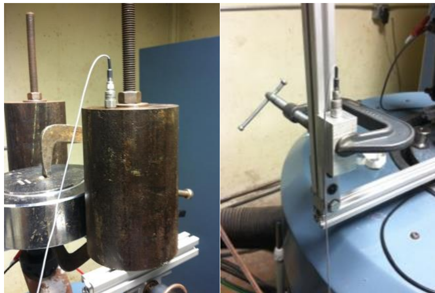
Figure 4.11 Accelerometer setup – second round testing.
