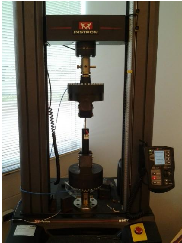
Figure 4.8: Tensile test for damper.
