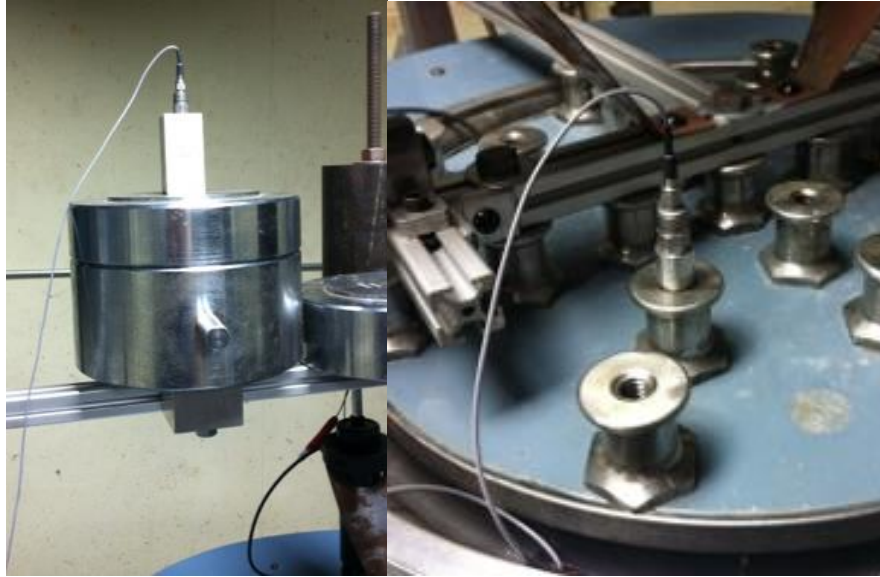
Figure 4.10: Accelerometer setup – first round testing.
