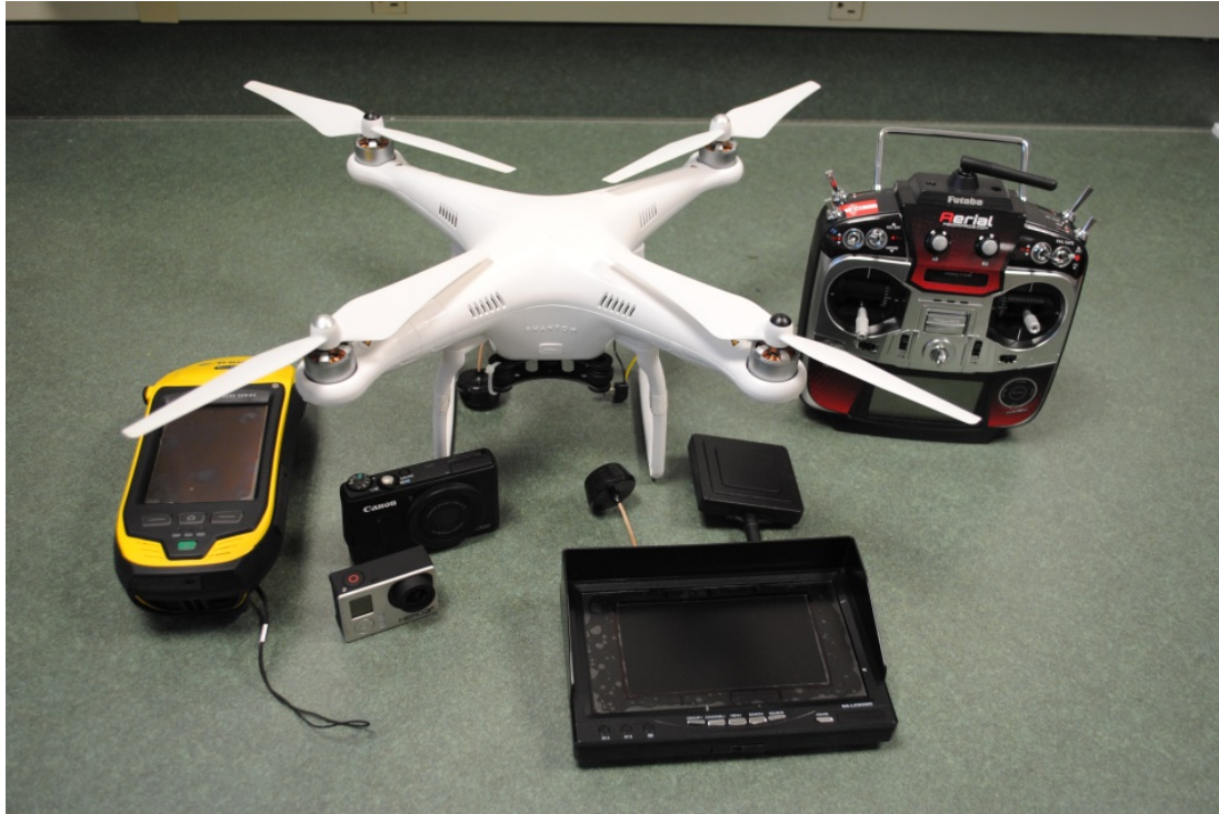
Figure 2. Equipment used for collecting aerial photographs from left to right: Trimble GeoXH DGPS unit, Go Pro Hero 4 digital camera, Canon S100 digital camera, DJI Phantom Vison 2 +, RX-LCD5802 LCD Monitor, and Futaba flight controller.
