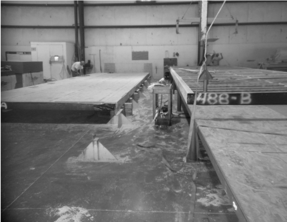
Figure 12. Squaring tables and jigs used in the manufacturing of modules (photo by author).
