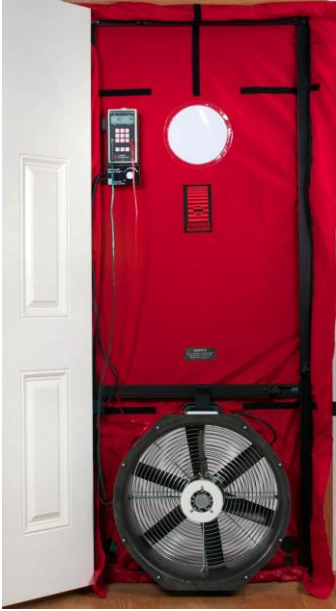
Figure 9. Blower door mock set-up.
