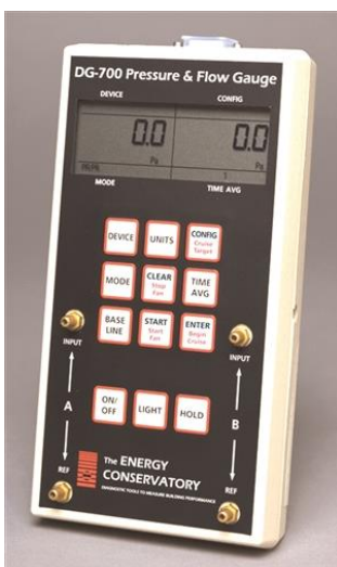
Figure 8. Hand-held manometer showing calibration to test conditions.
