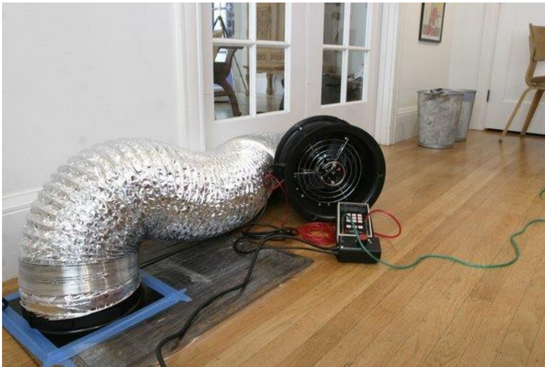
Figure 10. Duct blaster mock set-up.
