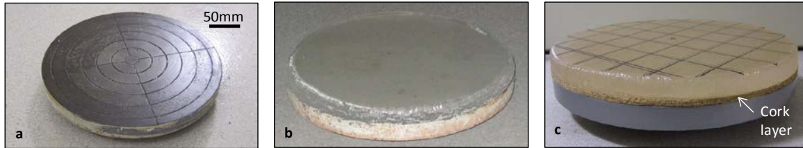
Figure 4-2: a. Steel substrate ( \text{Ø}=300 mm), and b. Tool A (22 mm pitch layer on steel substrate), c. Tool B (steel substrate, 6 mm cork layer and 22 mm of pitch).
