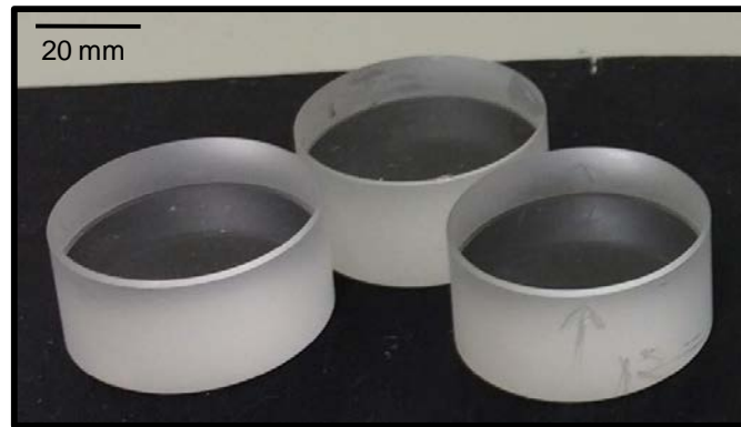
Figure 4-14: Fused Silica samples ( \varnothing = 25 mm) used in the polishing tests.
