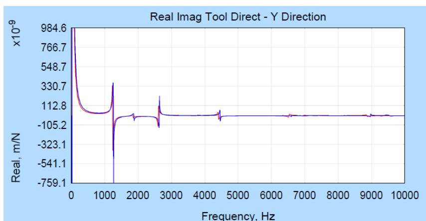
Figure 3-11: Test results (frequency response) for MS platen (blue) and the tool (red) made from MS platen.
