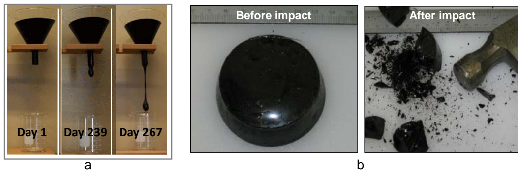
Figure 2-5: a. Pitch a very high viscous liquid, b. Brittle fracture resulted from an impact hit [7].
