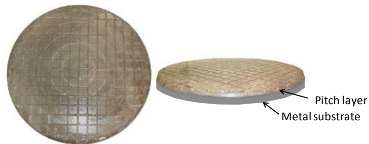
Figure 2-3: pitch tool with grooving [24].
