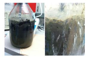
FIGURE 4.9: Foam formation during digestion
