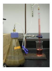
FIGURE 3.4: A photograph of the acid-brine gas displacement apparatus for measuring gas volume
