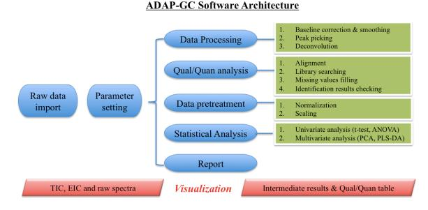
Figure 4.1. ADAP-GC software architecture
