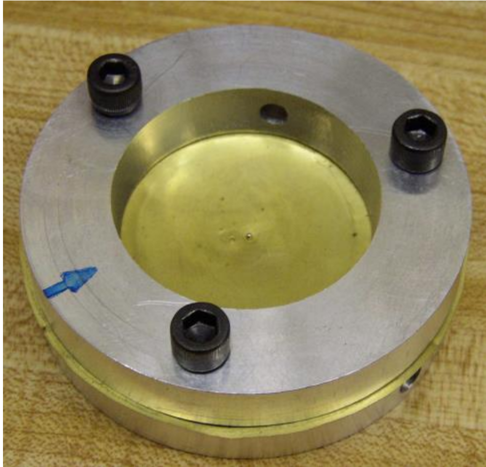
Figure 45: Ball holder for the RBT. Two big washers sandwich a sheet of shim, and an indentation is used for positioning the ball.
