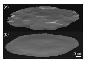
Figure 3.6: The upper (a) and lower (b) interfaces of InGaN QW layer reconstructed from APT experimental data. [10]
