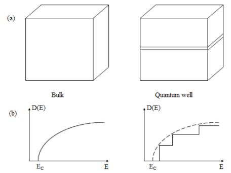
Figure 2.2: Schematic morphology (a) and density of states (b) in bulk semiconductor material and QW.
