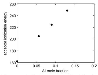
Figure A.1: Mg acceptor ionization energy vs. Al mole fraction in AlGaN [57].
