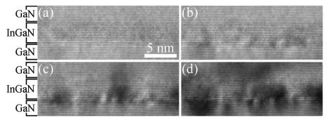
Figure 3.4: (0002) lattice fringe images showing strain contrast evolution in an  $In_{0.22}Ga_{0.78}N/GaN$  MQW after be exposed to a 200 kV electron beam flux of 35 A/ cm<sup>2</sup> after: (a) 20, (b) 220, (c) 420, and (d) 620 s [90].
