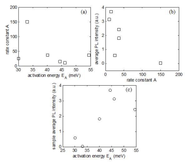
Figure 5.7: (a) first channel rate constant vs channel activation energy; (b) sample average intensity vs first channel rate constant(c) sample average intensity vs thermal activation energy  $E_A$ .
