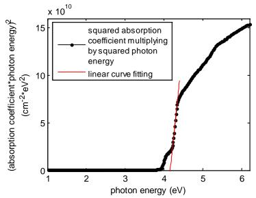
Figure A.6: Squared absorption coefficient multiplying by squared photon energy vs. photon energy. The intersection between the linear fitting line and the *x*-axis indicates the bandgap energy.
