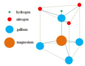
Figure A.2: Schematic diagram of the Mg-H bond in GaN. The hydrogen is located in the anti-bonding site, which is thought to be the most favorable place. [132]
