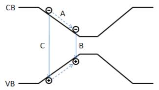
Figure 5.2: Explanation of red-blue-red shift of PL peak position as temperature increases.Process (A) shows the carriers relax down to the bottom of confining potential; process (B) shows the recombination at bottom of confining potential; and process (C) shows carriers recombine before reaching the bottom of the confining potential.
