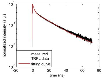
Figure 5.24: Measured TRPL spectrum for bright region in sample #7 and its fitting curve. The Adj. R-square of the fitting is 0.9973.
