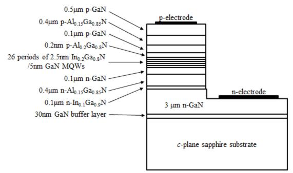
Figure 4.3: Structure of an InGaN MQWs laser diode [107].
