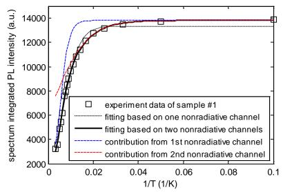
Figure 5.6: (Color) Spectrum integrated PL intensity as a function of temperature for sample #1 and the fitting curves to it.
