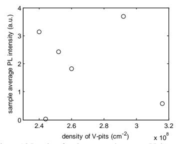
Figure 5.2 Density of v-pits vs. sample average PL intensity.
