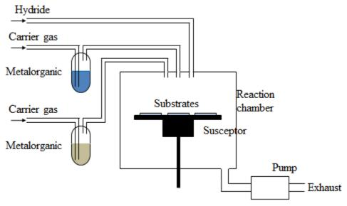
Figure 2.7: Schematic diagram of MOCVD.
