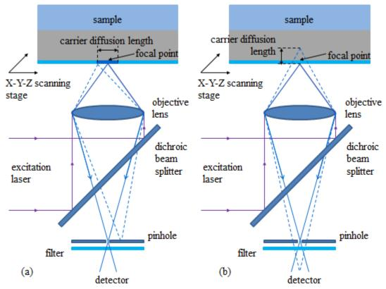
Figure 4.9: Working scheme of confocal laser scanning microscope.
