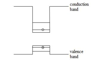
Figure 2.3: One electron and one hole form an exciton in QW.
