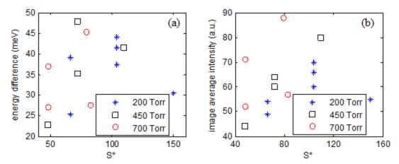
Figure 5.6: (a) Bandgap energy difference and (b) CLSM image average intensity as a function of effective gas speed (S<sup>\*</sup>) for sample #7 to sample #20. Note the highest intensity samples are at 450 Torr and 700 Torr.
