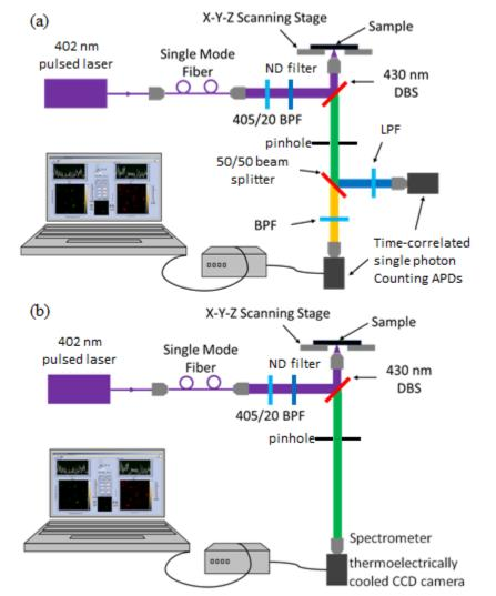
Figure 4.12: Schematic diagram of CLSM system for (a) spectrum measurements and (b) TRPL measurements.
