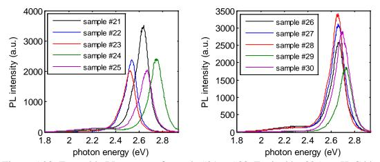
Figure 5.28: Ensemble PL spectra of sample #21 to #30. Excited by 325 nm HeCd laser.
