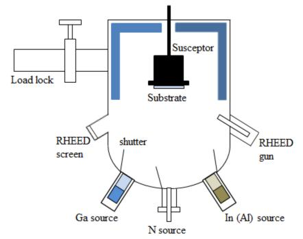
Figure 2.6: Schematic diagram of MBE. The RHEED (reflection high energy electron diffraction) gun and screen are used for in-situ monitoring the growth.
