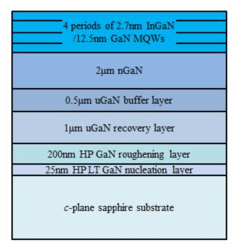
Figure 2.8: Structure of blue-emitting InGaN MQWs provided by Veeco Instruments Inc.
