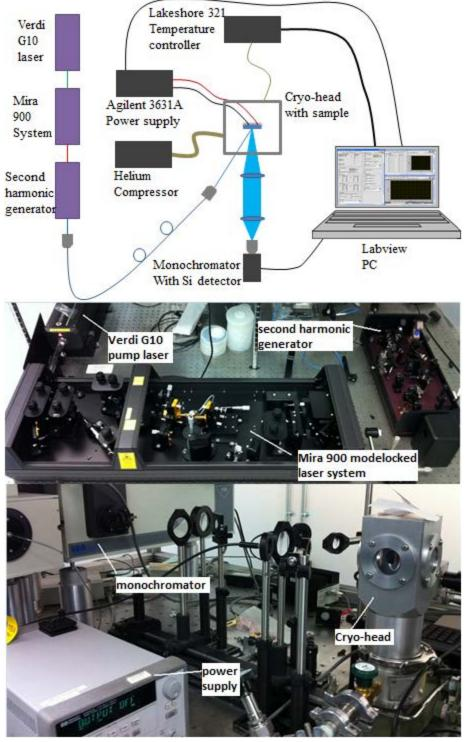
Figure 4.7: (Color) Schematic diagram and photo of low temperature PL system.
