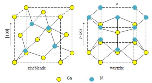
Figure 2.1: The zinc blende and wurtzite crystal structures of GaN. The zinc blende structure can be described using the edge length a, while the hexagonal wurtzite structure can be described using the edge length a of the basal hexagon and the height c of the hexagonal prism.
