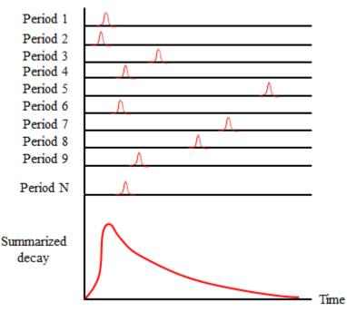
Figure 4.13: Principle of TCSPC.
