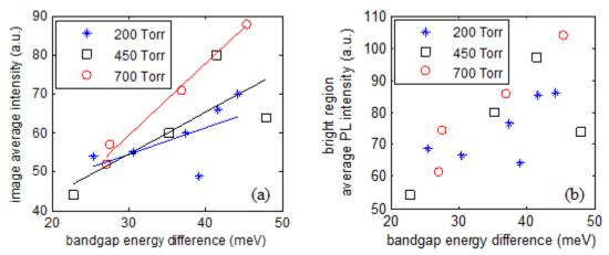
Figure 5.4: (a) CLSM image average intensity vs. bandgap energy difference between bright region and dark region, solid lines show the linear fitting to the data, the adj. Rsquare for the fitting are 0.22 for 200 Torr data, 0.38 for 450 Torr data, and 0.98 for 700 Torr data; (b)bright region average PL intenisty vs. bandgap energy difference between bright region and dark region.
