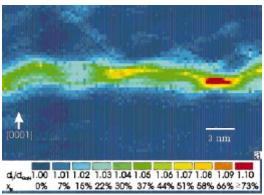
Figure 3.3: Color-coded map of the local indium concentration in blue emitting InGaN/GaN QW, calculated based on TEM lattice fringe images showing strain contrast. An inhomogeneous indium distribution is observed in the quantum well varying between 20% and 80% [26].
