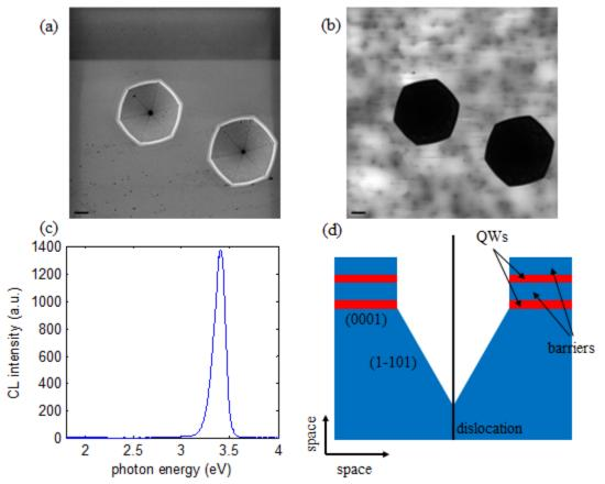
Figure 5.17: (a) SEM image of sample #14 showing surface morphology, large V-pits can be seen; (b) CL image showing intensity distribution at 459 nm, taken at the same place as SEM image; (c) CL spectrum taken at the sidewall of the V-pit; (d) model of the Vpits showing no MQWs on the sidewalls. The SEM and CL images are 15µm×15µm.
