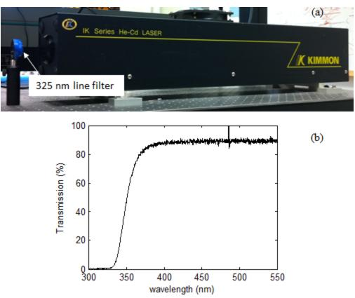
Figure 4.1: (a) Photo of He-Cd laser; (b) the transmission spectra of the line filter and cutoff filter used in the He-Cd laser.
