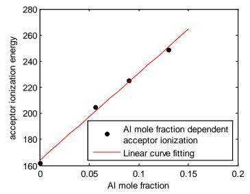
Figure A.10: The relation between acceptor ionization energy and Al mole fraction, replotted from ref [57], and the linear fitting for it. The adjusted R-square of the fitting is 0.9927.
