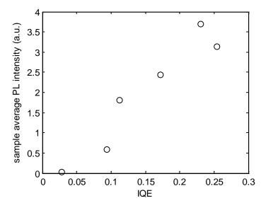
Figure 5.1: Room temperature sample average PL intensity vs. IQE.
