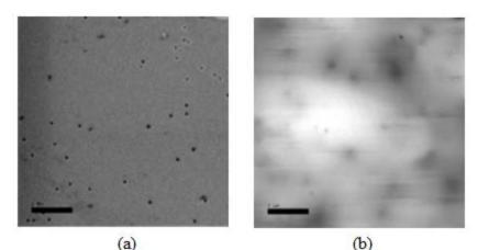
Figure 5.18: SEM image (a) and CL image at 445 nm (b) of the same place on sample #14. Both images are 5µm×5µm.
