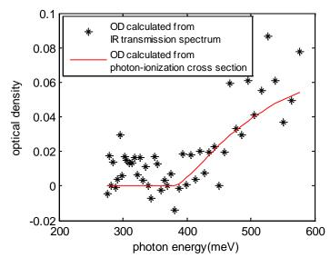
Figure A.9: OD calculated by both Equation (A.3) and Equation (A.4), the R-square for the fitting is 0.6155.
