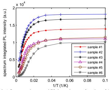
Figure 5.5: (Color) Spectrum integrated PL intensity as a function of 1/T for InGaN/GaN MQW samples.
