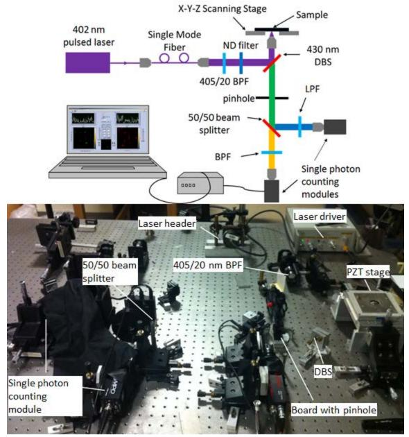
Figure 4.10: Schematic diagram and photo of CLSM system for imaging.
