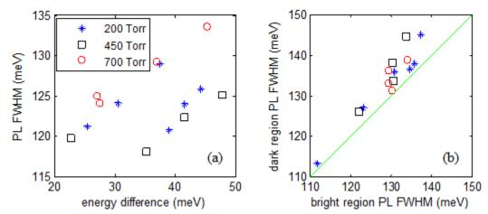
Figure 5.19: (a) FWHM of ensemble PL vs. bandgap energy difference between bright region and dark region; (b) PL FWHM in dark regions vs. PL FWHM in bright regions, solid line shows the place where the two FWHMs equal. InGaN MQWs grown under different pressure are marked with different symbols.
