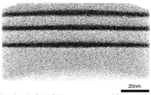
Figure 3.5: Image showing InGaN QWs, reconstructed from APT data. Gallium atoms are shown as gray and indium atoms as black. Other atoms are omitted for clarity. [10]
