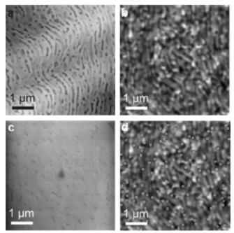
Figure 3.8: (a) AFM image of an annealed InGaN epilayer. Interlinking InGaN strips with GaN troughs between them can be seen; (b) CL image of an InGaN QW which is grown and annealed under the same conditions as the InGaN epilayer. Bright emission from the InGaN strips can be seen; (c) SEM image recorded at the same time with the CL image, showing a lot of V-pits; (d) V-pits observed in (c) are marked on the CL image as white rings. [100]
