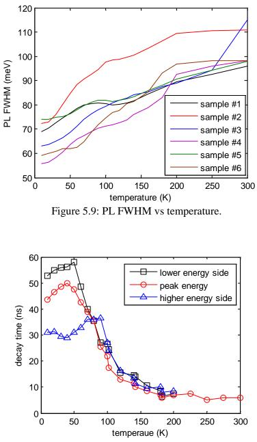
Figure 5.10: PL lifetime vs. temperature for the InGaN/GaN MQW structure. Note that for T<70 K the lifetime is smaller at lower energy side, while for T>70 K there is no difference between those three lifetimes. This 70 K is also the temperature at which the InGaN PL peak energy turns from redshift to blueshift with increasing temperature. Replotted from [120].
