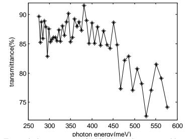
Figure A.7: Transmission spectrum of AlGaN sample, measured by OPO/OPA and power meter.
