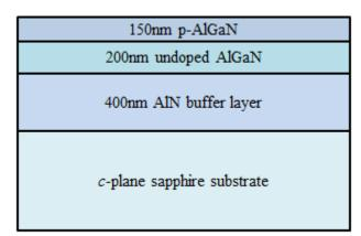
Figure A.3: Structure of p-AlGaN sample provided by Sensor Electronic Technology Inc.
