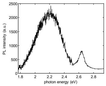
Figure 5.31: PL spectrum of sample #21 at yellow dot. The primary peak at 550 nm indicates yellow luminescence. The secondary peak at around 460 nm is from bandedge emission light which is not totally blocked by the LPF.
