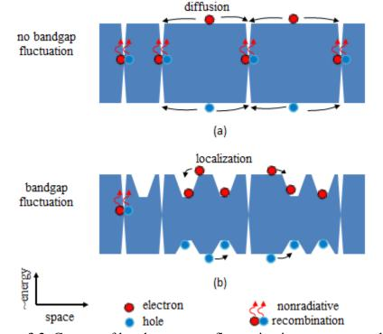
Figure 3.2: Cartoon of bandgap energy fluctuation in nanometer scale.
