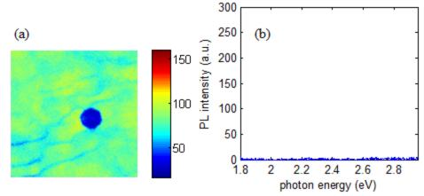
Figure 5.16: (a) CLSM image of sample #14 taken with 445/40 nm BPF, showing a very large V-pit with the size of about 4  $\mu$ m, the image is 20 $\mu$ m×20 $\mu$ m in size; (b) PL spectrum taken at the sidewall of the V-pit.
