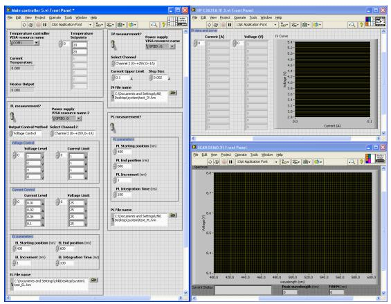
Figure 4.8: User interface of the Labview program that controls the low temperature PL/EL/IV system.
