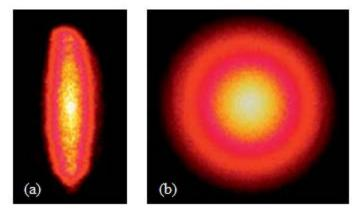
Figure 4.11: Beam shape at the output of LD (a) and optical fiber (b) [110].
