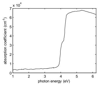
Figure A.5: Absorption coefficient spectrum of the AlGaN sample.
