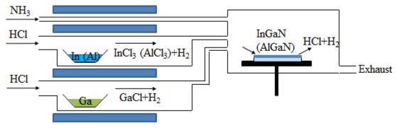
Figure 2.5: Schematic diagram of HVPE [74].
