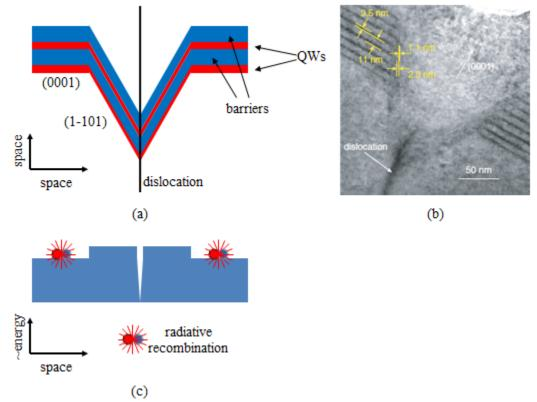
Figure 3.7: Schematic diagram (a), TEM image [97] (b), and bandgap diagram (c) of Vpits in InGaN MQWs.
