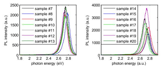
Figure 5.3: Ensemble PL spectra of samples #7 to #20. Excited by 325 nm HeCd laser and measured by OceanOptics USB2000.
