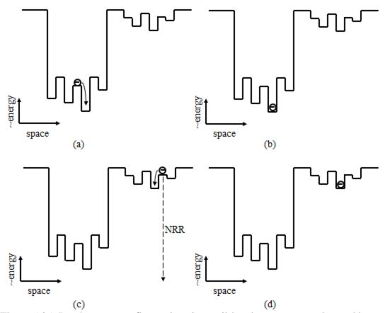
Figure 5.25: Bandgap energy fluctuations in small-bandgap-energy region and largebandgap-energy region, carrier localization in local weakly localized states (a)(c), and carrier localization in local strongly localized states (b)(d).
