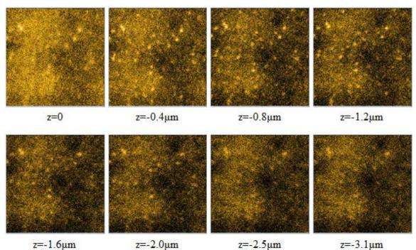
Figure 5.32: z-scan of with 538 nm LPF. z=0 means the focal point is at the sample surface; z=-3.1 μm means the focal point is 3.1 μm inside the sample.
