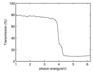
Figure A.4: Transmission spectrum of AlGaN sample, measured by UV-VIS-IR spectrophotometer.
