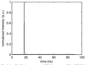
Figure 5.23: IRF of the CLSM system and TRPL system. The FWHM of the IRF is 385 ps.
