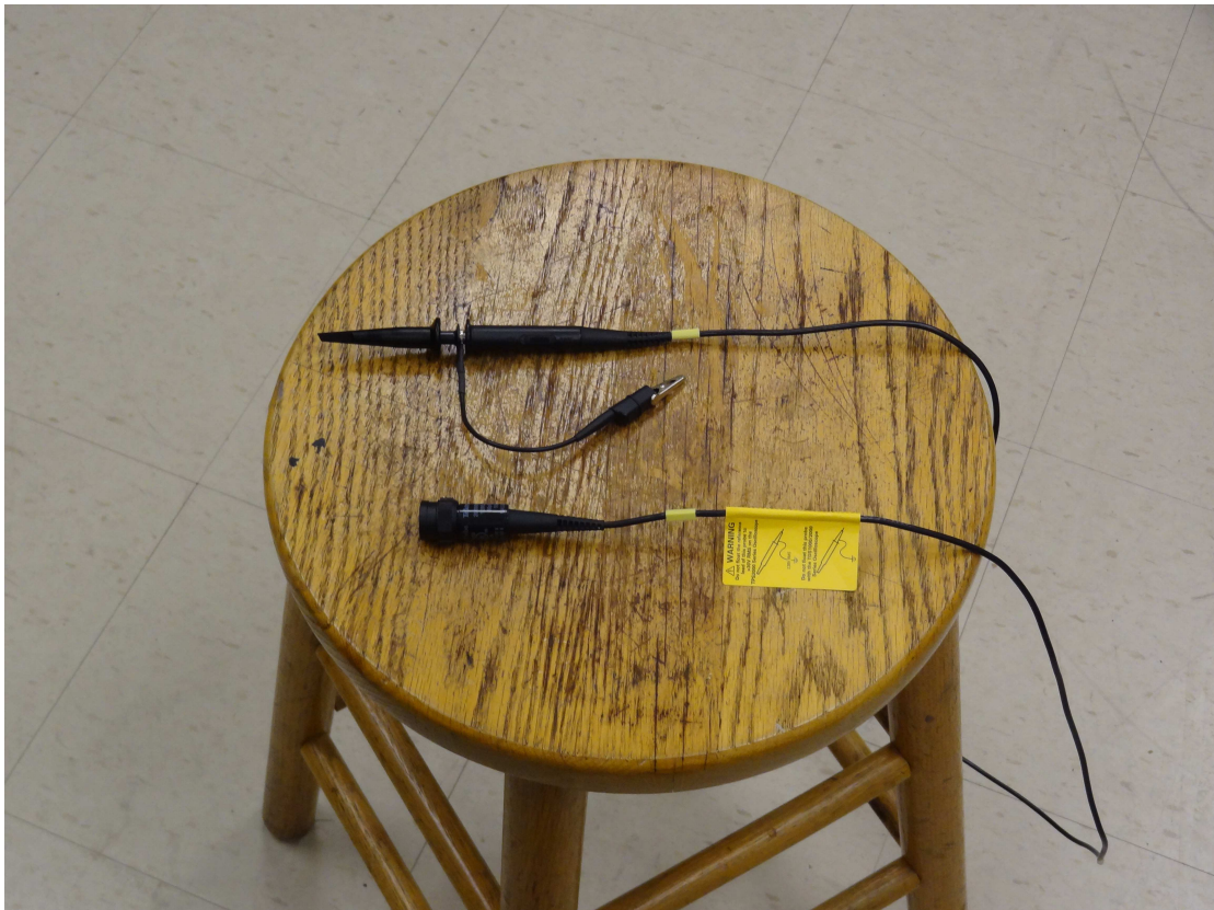
Figure 167: a picture of an oscilloscope probe utilized to acquire differential measurements within the laboratory
