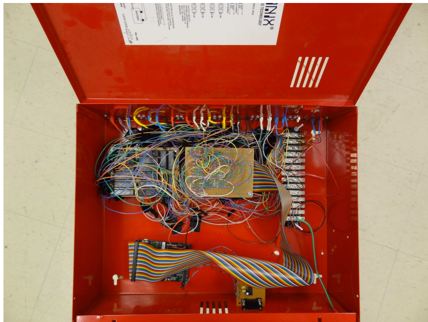
Figure 391: a picture of the internal workings of medusa, the custom-designed 40 to 1 remote-controlled analog channel multiplexer
