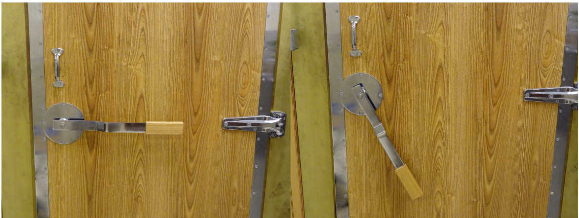
Figure 71: (left) partially shielded rf enclosure with external power, (right) fully shielded rf enclosure without external power
