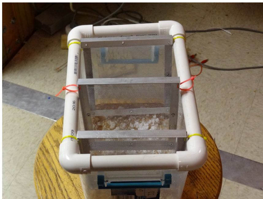
Figure 447: a picture of a custom fabricated aluminum screen testing apparatus
