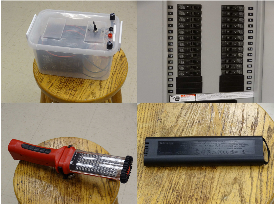
Figure 189: (top left) a picture of the custom built \pm 12\text{v} battery box utilized to power electrical circuitry for low power rf shielded room operations, (top right) a picture of the electrical breaker utilized to isolate the rf shielded room from the power grid, (bottom left) a picture of the battery-operated lantern utilized to provide illumination for low power rf shielded room operations, (bottom right) a picture of the tektronix tps2024 oscilloscope battery utilized for low power rf shielded room operations
