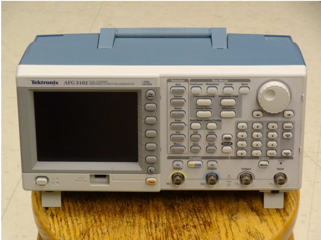
Figure 181: a picture of the tektronix afg3102 signal generator
