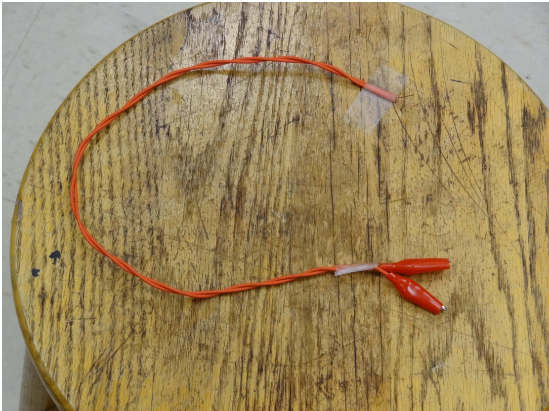
Figure 174: a picture of how interconnection wires were twisted when utilized to obtain a laboratory measurement
