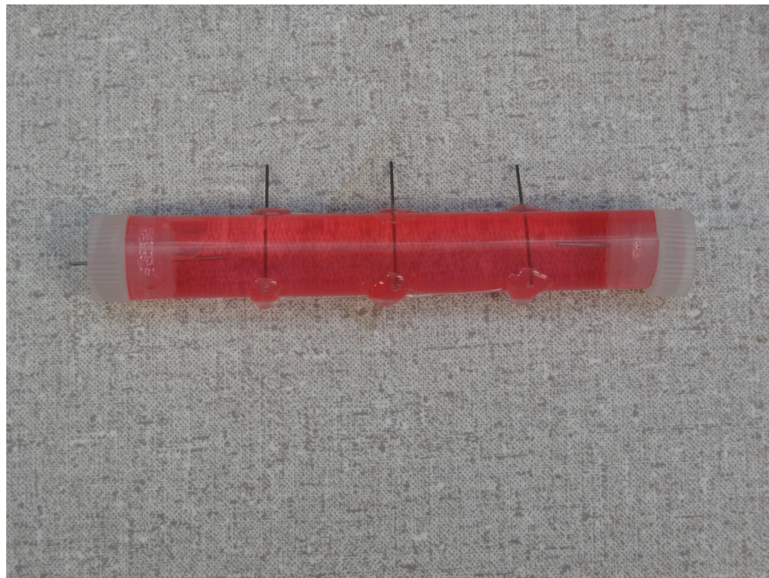
Figure 409: a picture of the testing apparatus developed to electrically characterize aqueous sodium chloride
