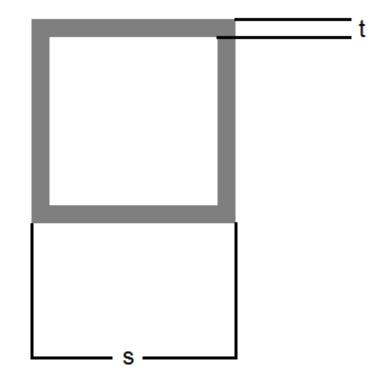
Figure 7.2: Cross section of the 200mm aluminum tube
