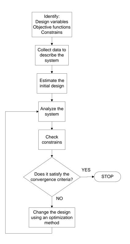
Figure 1.1: Optimum design process
