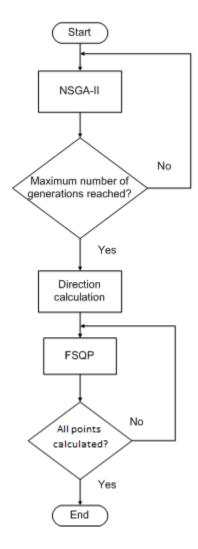
Figure 5.21: Flowchart of the second hybrid algorithm
