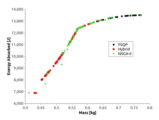
Figure 7.10: Comparison of the constrained tube solutions
