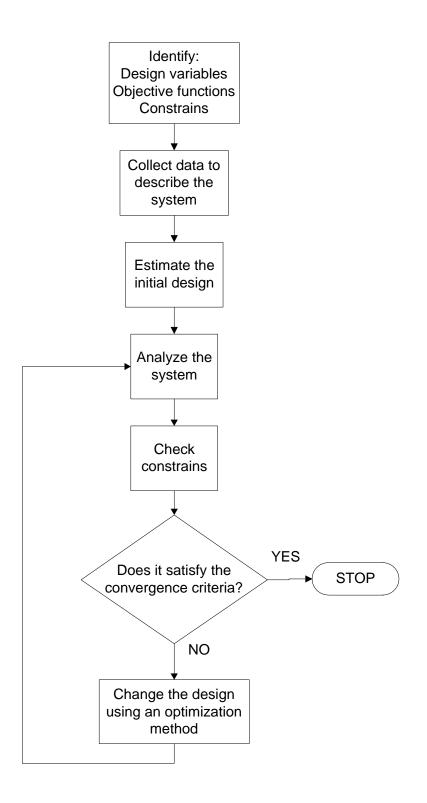
Figure 2.2: An optimum design process
