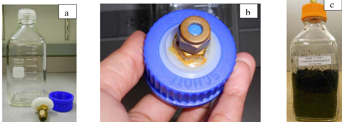
Figure 7.1: (a) 1 L capped glass bottles, (b) NPT Swagelok fittings, (c) Bottles with inoculum and test specimen
