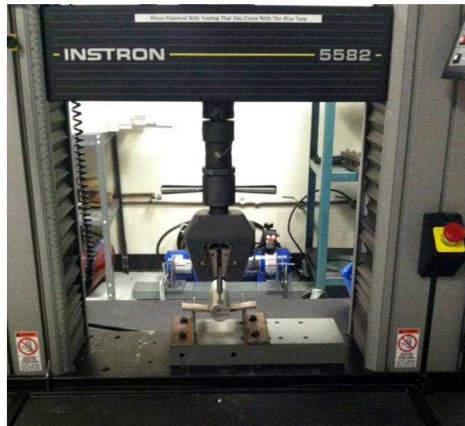
Figure 3.12: Instron loaded with a composite specimen for testing in flexural mode
