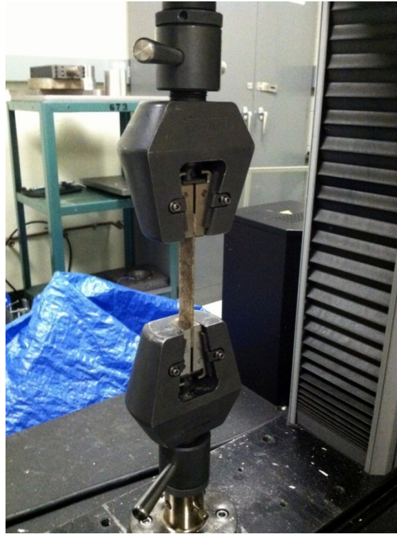
Figure 3.11: Instron loaded with a composite specimen for testing in tensile mode
