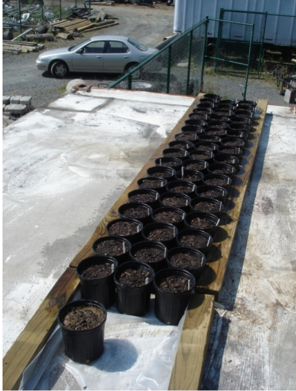
Figure 12: Gypsum drywall amended tall fescue pot experiment
