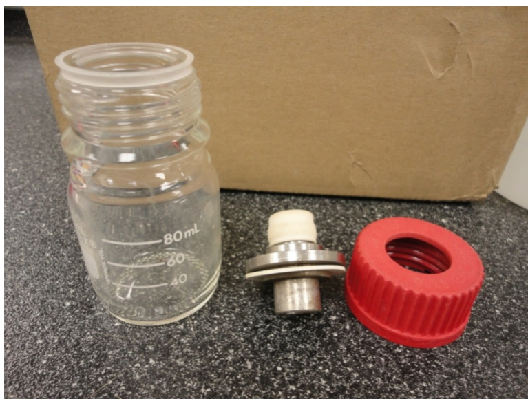
Figure 20: Bottle and cap used in the GC method
