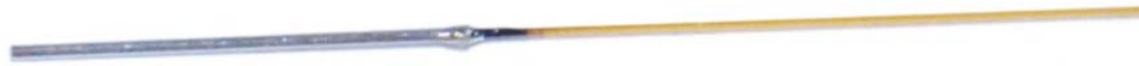
Figure 5.2: Photograph of \sim 350 \mu\text{m} OD, 10 mm long stainless steel tube glued to 150 \mu\text{m} core diameter trunk fiber.
