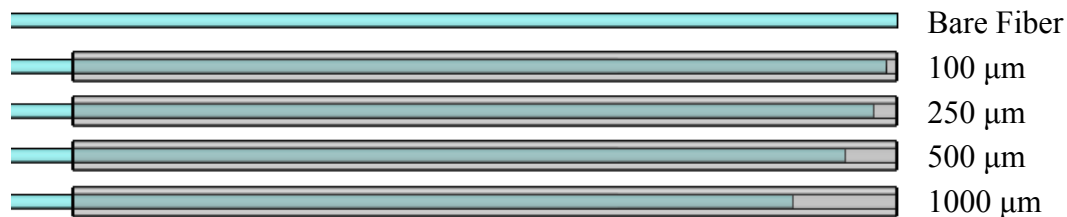
Figure 5.3: Scale representation of five fiber tips tested based on fiber recession distance. Length of stainless steel tube: 10 mm.
