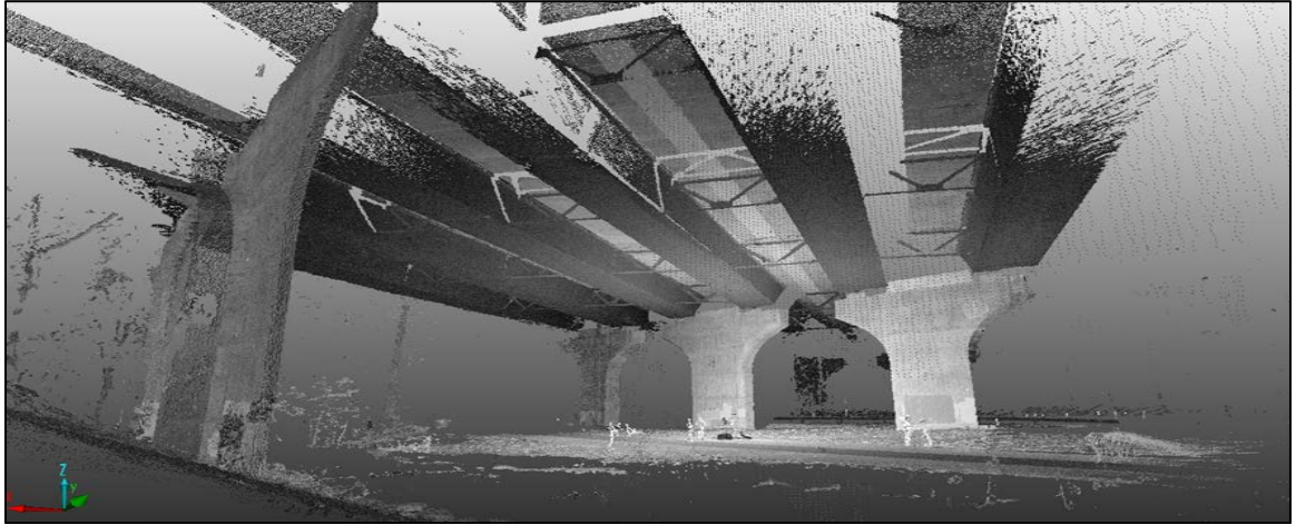
Figure 3.2 3D reconstruction of LiDAR scanning data of a highway bridge
