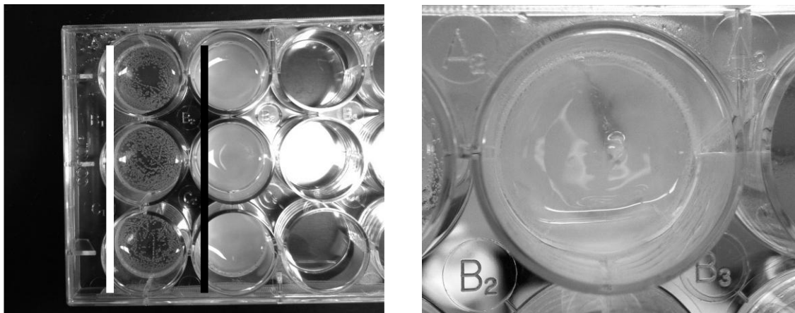
FIGURE 3.7 In a standard 12-well plate (LEFT), normal medium treated, clear collagen gel (white line marked) and 5% PFC-medium treated collagen gel for 3 days (black line marked), where a closer view shows that PFC sediment gives collagen a cloudy look (RIGHT).
