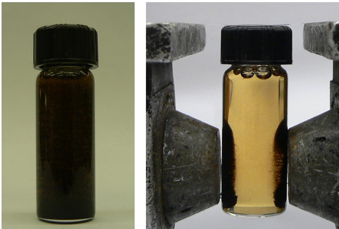
Figure 3.3.: Demonstration of magnetic properties of \text{CoFe}_2\text{O}_4 -Pd linked NPs. The image on the left shows a concentrated solution of the NPs. The image on the right shows the same solution immediately after placing it in a magnetic field.
