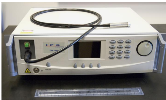
Figure 3.3: Compact, portable, and tunable wavelength of 1850 nm to 1880 nm Thulium fiber laser was used in the nerve stimulation studies.
