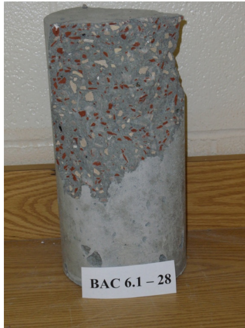
Figure C-11: Test specimen used for compressive strength, modulus of elasticity, and Poisson's ratio testing, RBMAC mixture BAC 6.1, 28 day tests.
