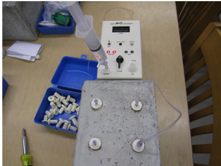
Figure 6-6: Water permeability testing using the Poroscope Plus equipment.
