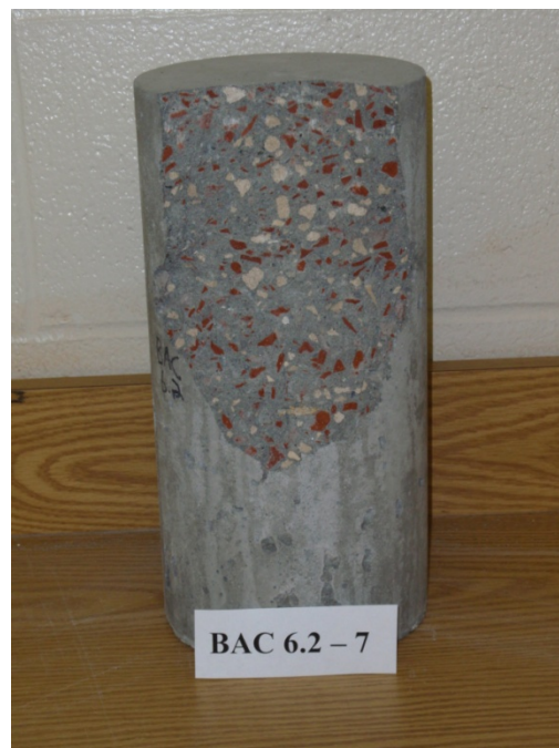
Figure C-14: Test specimen used for compressive strength, modulus of elasticity, and Poisson's ratio testing, RBMAC mixture BAC 6.2, 7 day tests.
