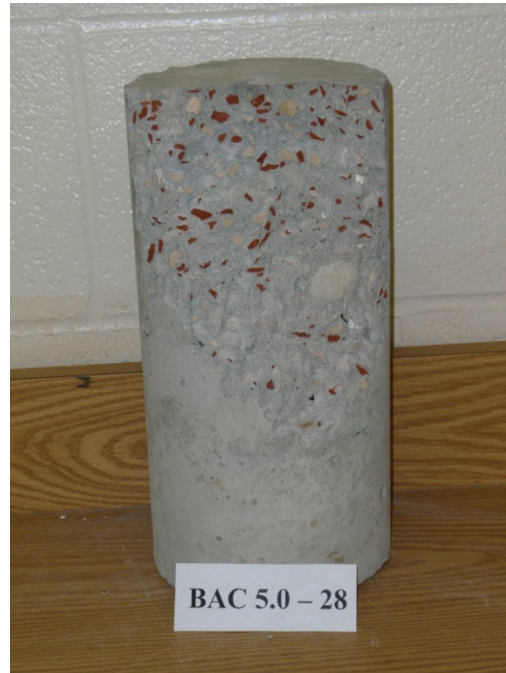
Figure C-3: Test specimen used for compressive strength, modulus of elasticity, and Poisson's ratio testing, RBMAC mixture BAC 5.0, 28 day tests.
