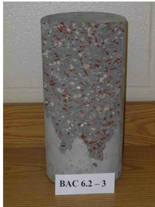
Figure C-13: Test specimen used for compressive strength, modulus of elasticity, and Poisson's ratio testing, RBMAC mixture BAC 6.2, 3 day tests.
