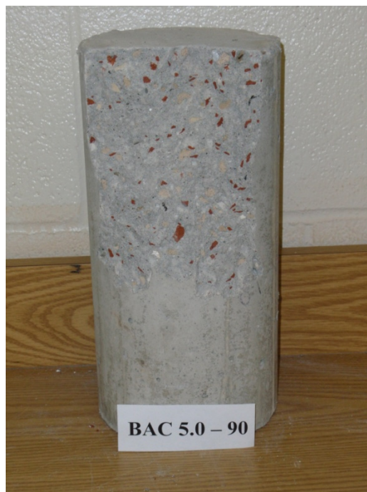
Figure C-4: Test specimen used for compressive strength, modulus of elasticity, and Poisson's ratio testing, RBMAC mixture BAC 5.0, 90 day tests.
