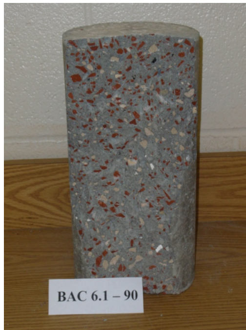
Figure C-12: Test specimen used for compressive strength, modulus of elasticity, and Poisson's ratio testing, RBMAC mixture BAC 6.1, 90 day tests.
