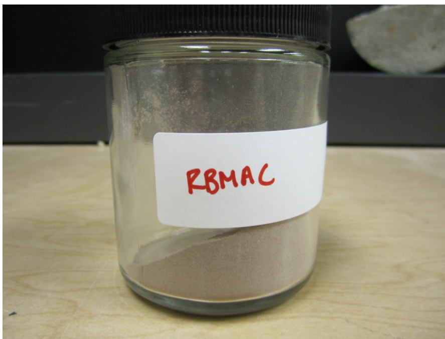
Figure C-27: Sample of crushed RBMAC (mixture BAC 6.2) used for heat capacity testing.
