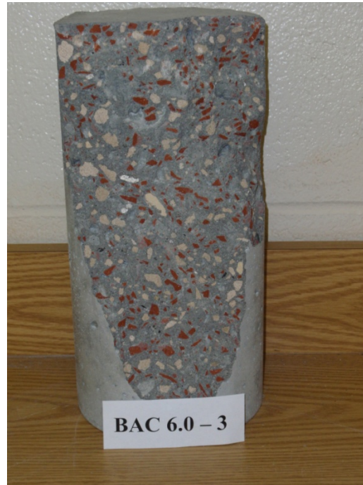
Figure C-5: Test specimen used for compressive strength, modulus of elasticity, and Poisson's ratio testing, RBMAC mixture BAC 6.0, 3 day tests.
