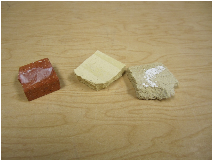
Figure A-3: Test specimens used for thermal conductivity testing.
