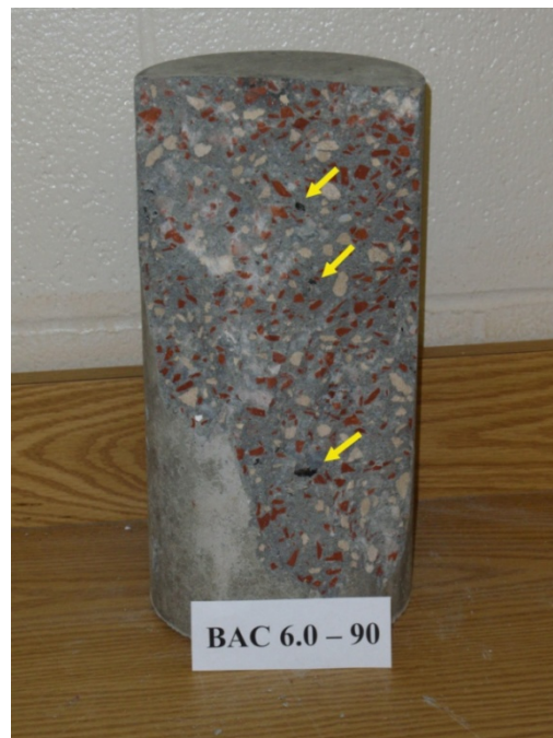
Figure 6-17: Contaminant particles are visible in the fractured surface of a compressive strength test cylinder.
