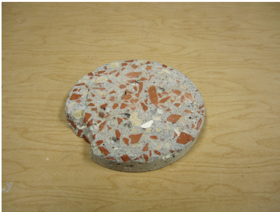
Figure C-25: Test specimen prepared from BAC 6.2 used for thermal conductivity testing.
