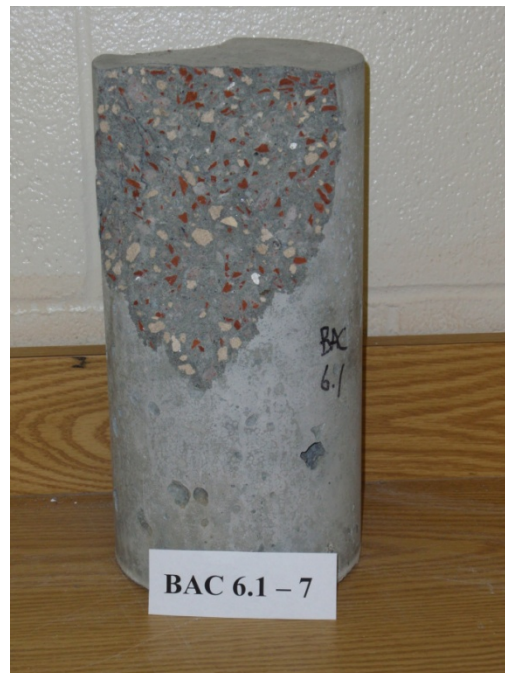
Figure C-10: Test specimen used for compressive strength, modulus of elasticity, and Poisson's ratio testing, RBMAC mixture BAC 6.1, 7 day tests.
