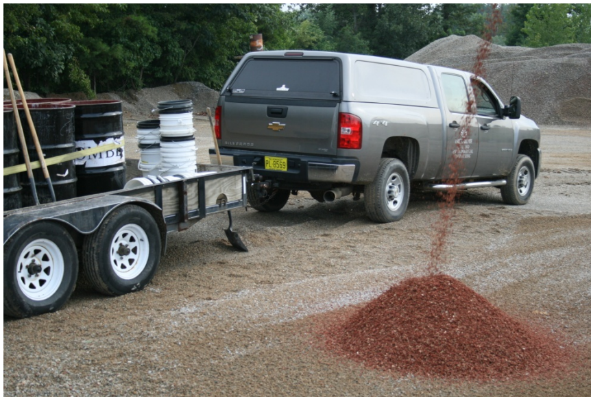
Figure 3-6: After falling from the conveyor belt, recycled brick masonry aggregate was shoveled into barrels and returned to UNC Charlotte laboratories.
