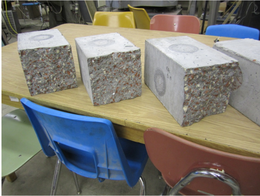
Figure C-19: Typical test specimens used for modulus of rupture testing, and subsequently, abrasion resistance testing.
