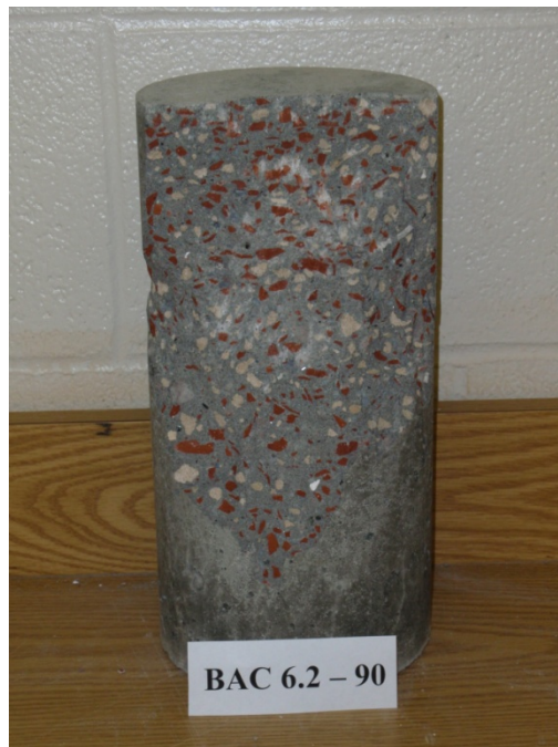
Figure C-16: Test specimen used for compressive strength, modulus of elasticity, and Poisson's ratio testing, RBMAC mixture BAC 6.2, 90 day tests.
