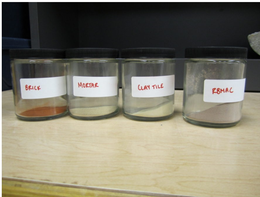
Figure C-28: Samples of crushed brick, mortar, clay tile, and RBMAC used for heat capacity testing.
