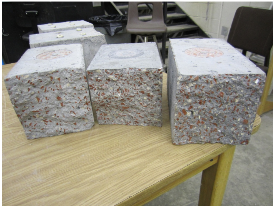
Figure C-31: Typical test specimens used for abrasion resistance testing (three specimens in front of photo) and air and water permeability testing (two specimens in rear of photo).
