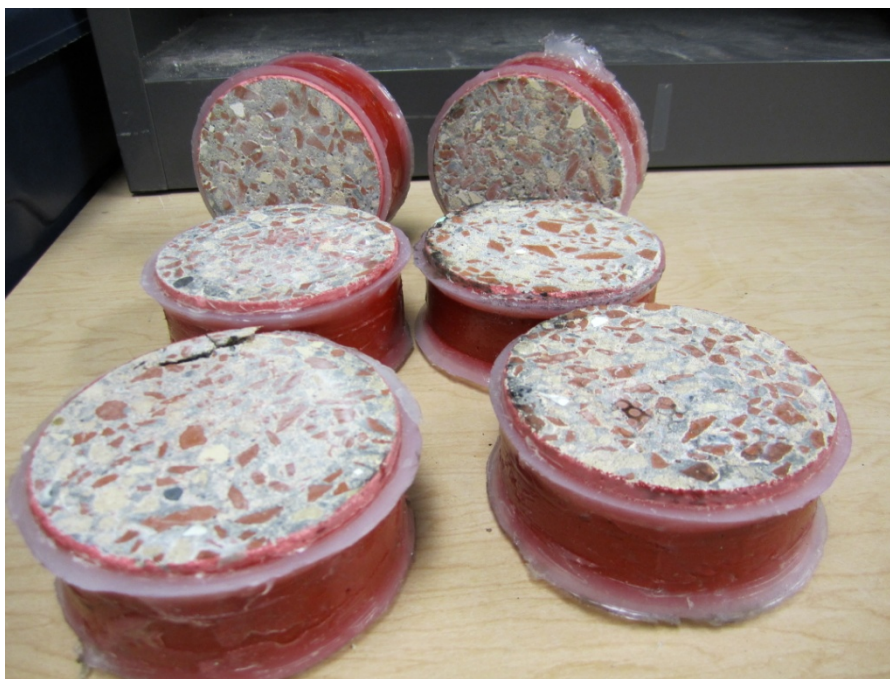
Figure C-32: Typical test specimens after rapid chloride ion permeability testing.
