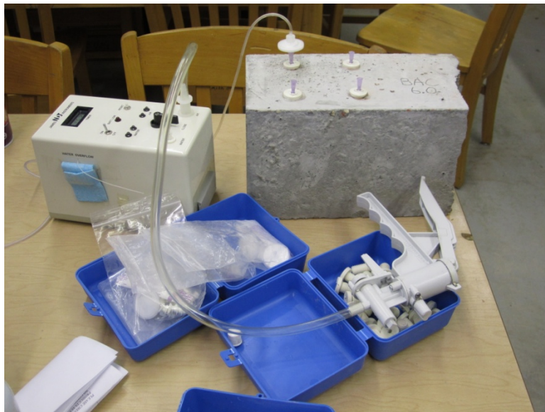
Figure 6-5: Air permeability testing using the Poroscope Plus equipment.
