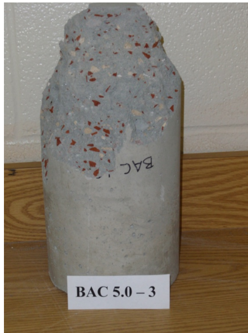
Figure C-1: Test specimen used for compressive strength, modulus of elasticity, and Poisson's ratio testing, RBMAC mixture BAC 5.0, 3 day tests.
