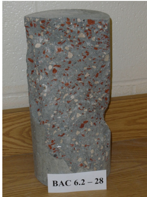
Figure C-15: Test specimen used for compressive strength, modulus of elasticity, and Poisson's ratio testing, RBMAC mixture BAC 6.2, 28 day tests.
