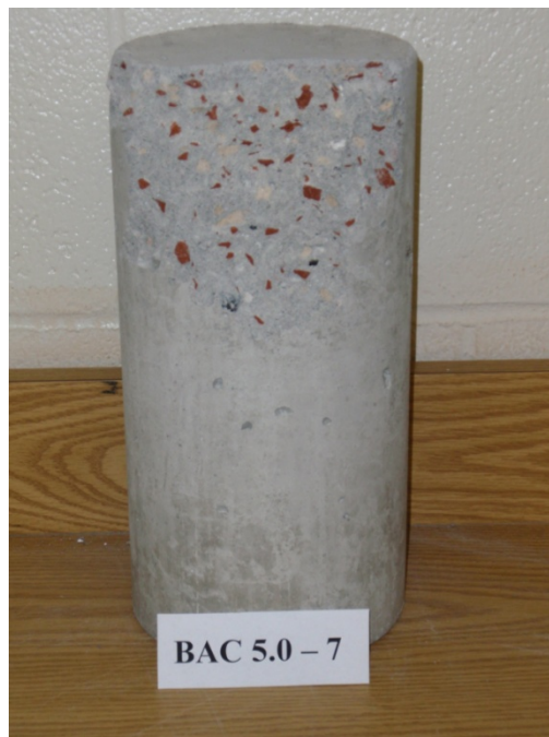
Figure C-2: Test specimen used for compressive strength, modulus of elasticity, and Poisson's ratio testing, RBMAC mixture BAC 5.0, 7 day tests.
