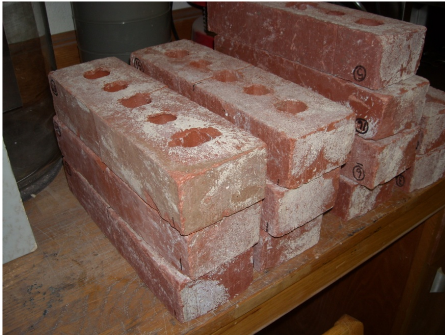
Figure A-1: Whole brick specimens.
