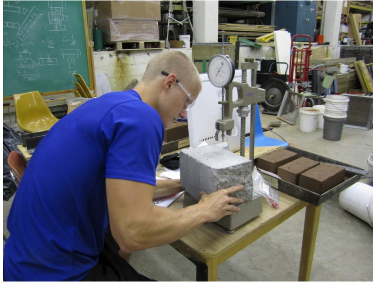
Figure 6-8: Apparatus used to determine the depth of abrasion.
