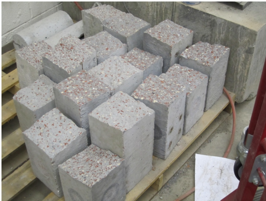
Figure C-20: Typical test specimens used for modulus of rupture testing, and subsequently, abrasion resistance testing and air and water permeability testing.
