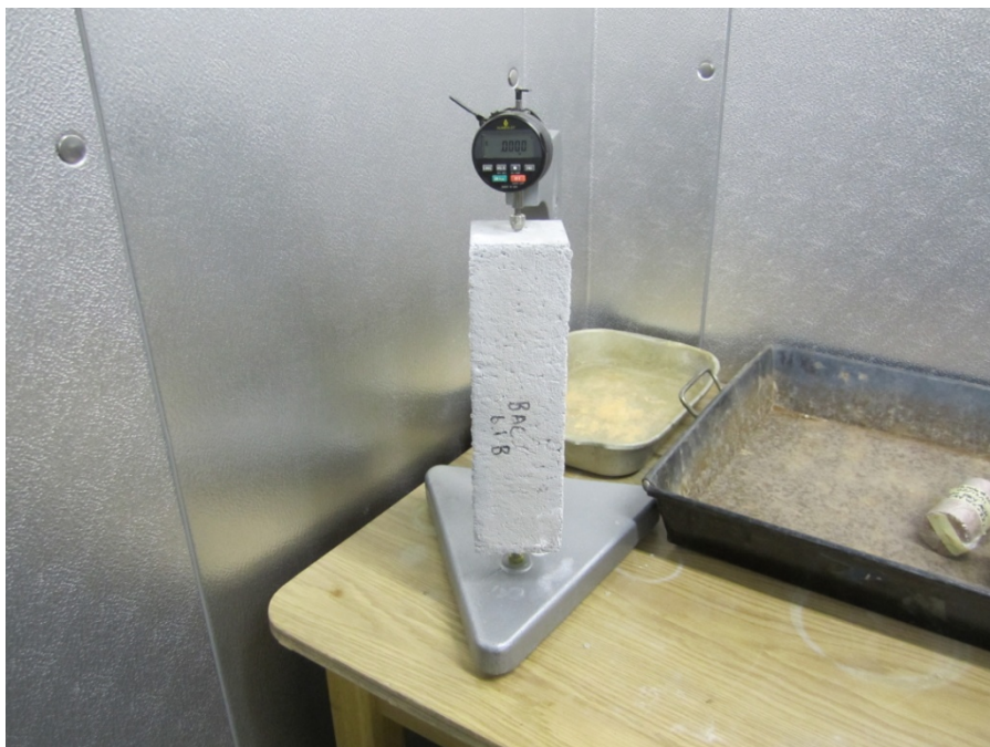
Figure C-24: Length measurement of drying shrinkage test specimen.
