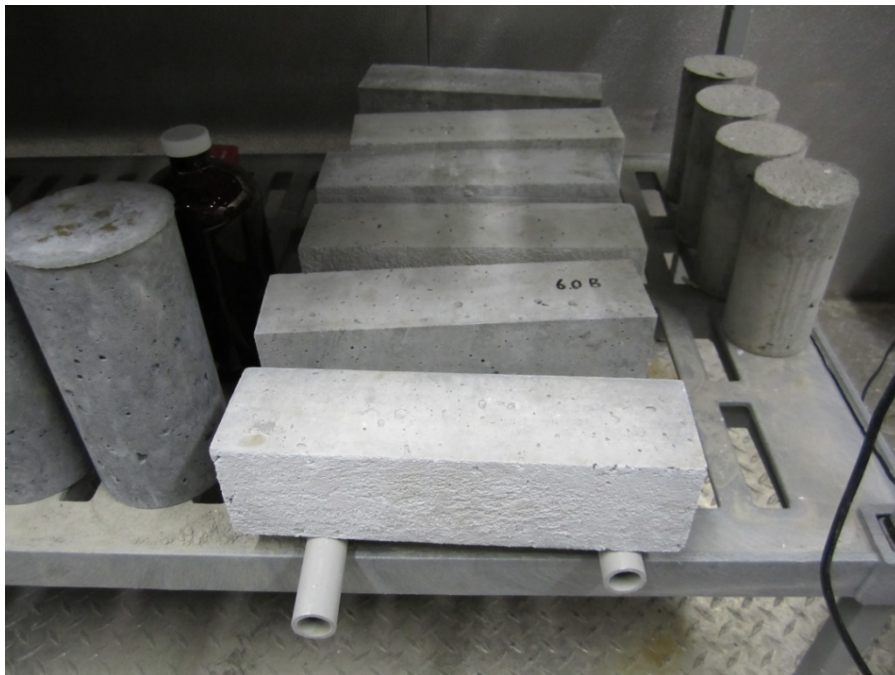
Figure C-23: Drying shrinkage test specimens (beams).
