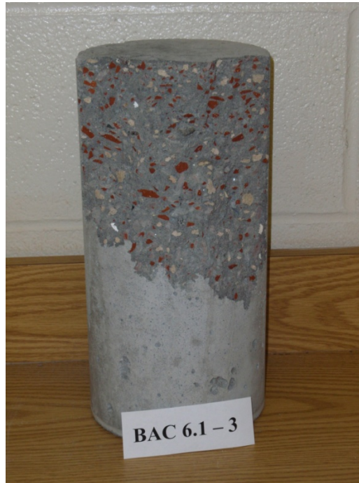
Figure C-9: Test specimen used for compressive strength, modulus of elasticity, and Poisson's ratio testing, RBMAC mixture BAC 6.1, 3 day tests.
