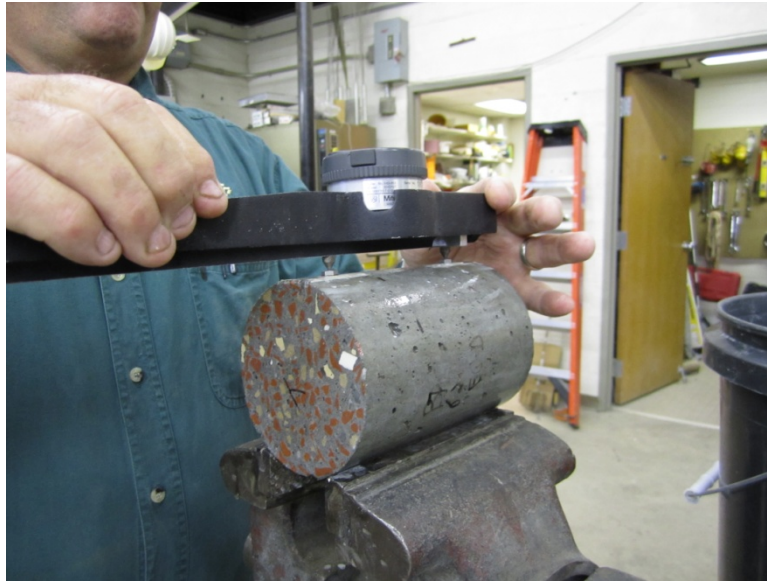
Figure 6-2: Mechanical strain gage used to measure length change of cylinder during testing to determine coefficient of thermal expansion.
