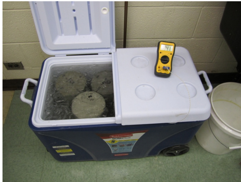
Figure 6-12: Conditioning of test specimens for surface resistivity testing at low temperatures.
