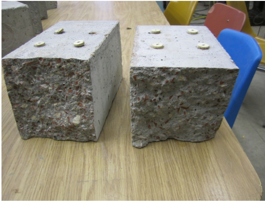
Figure C-30: Typical air and water permeability test specimens after testing.
