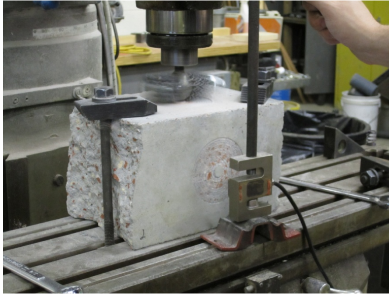
Figure 6-7: Abrasion testing using the rotary cutter method.
