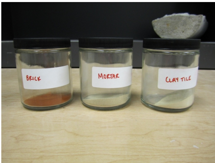
Figure A-7: Samples of crushed brick, mortar, and clay tile, for heat capacity testing.
