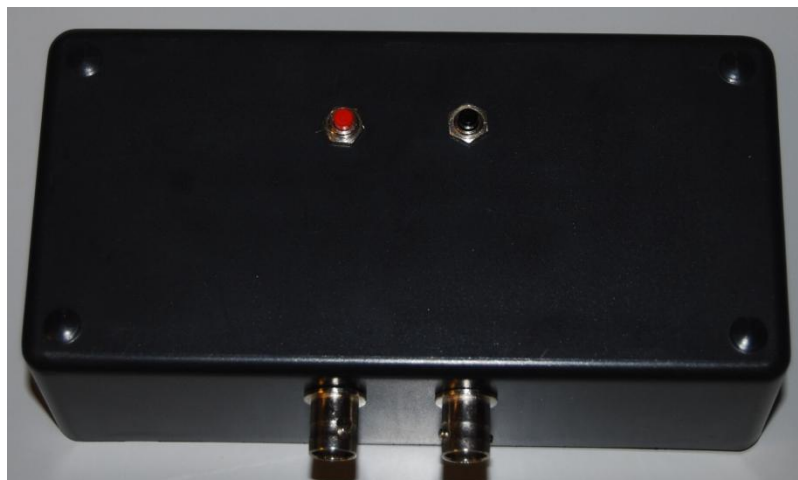
Figure A-6. Project box housing Renesas microcontroller board with BNC connectors
