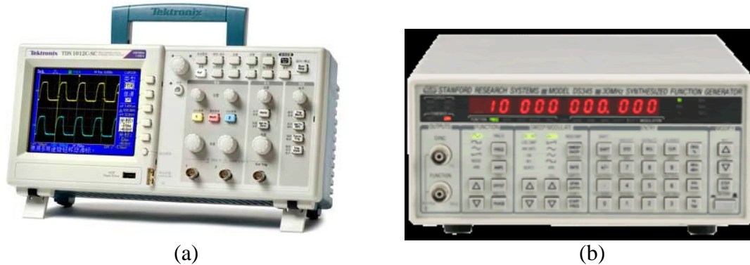
Figure A-4. (a) Tektronix digital oscilloscope, (b) Stanford Research Systems signal generator.
